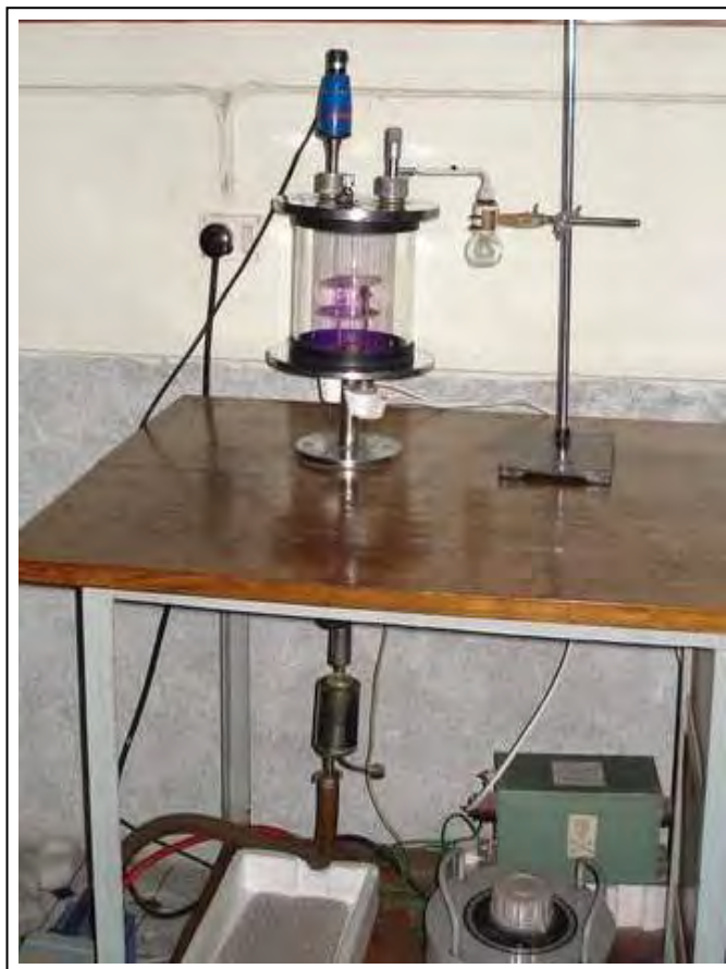
Fig. 3.3: The plasma polymerization set-up
