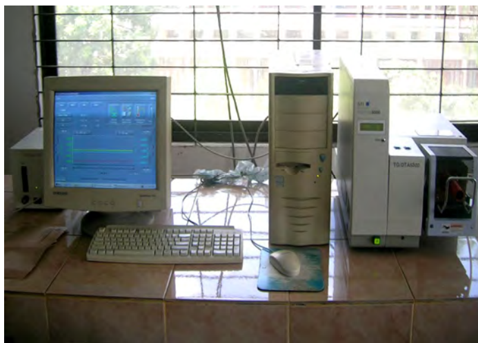
Fig.4.9: A coupled differential thermal analyzer and thermogravimetric analyzer.
