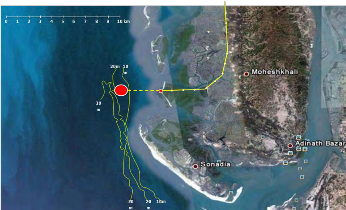
Figure 5.1: Tentative sea island location and Pipe Line route for LNG (Source- LNG project cell, Petobangla)
