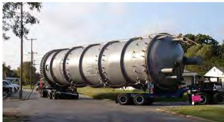
Figure 3.6: LNG Boil off gas (BOG) condenser (Source- Boardman)
