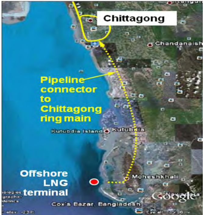
Figure 5.2: Proposed pipeline from south of Chittagong to Moheshkhali Island (Source- LNG project cell, Petobangla)
