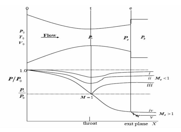
Figure 4.4: Pressure profile for isentropic flow in a converging-diverging nozzle [15]
