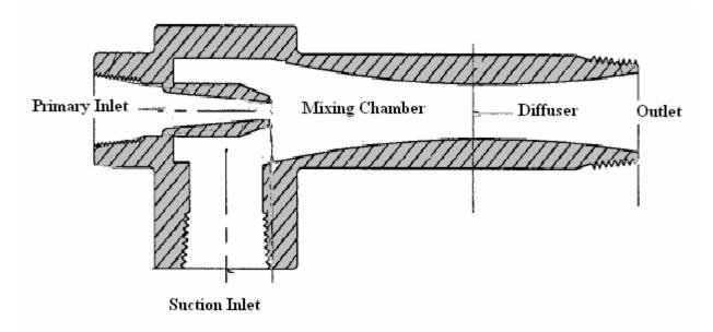
Figure 2.1: Cross sectional view of a typical liquid jet pump
