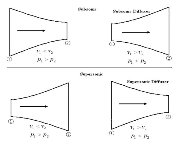
Figure 4.5: Nozzle and diffuser shapes for subsonic flow and supersonic flow
