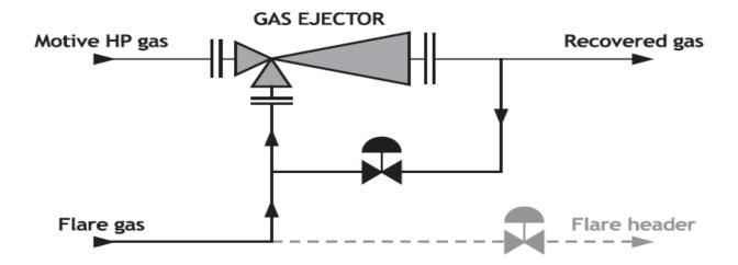
Figure 2.5: Ejector flare gas recovery system
