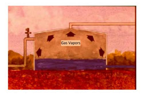
Figure 1.1: Tank Operations, as the condensate resides in the tanks, it gives off vapors,
