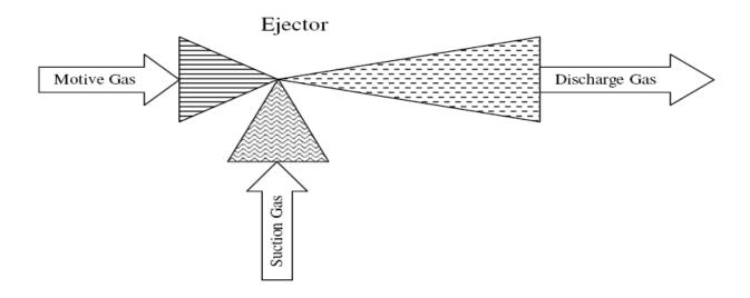
Figure-2.3: Schematic of a Gas Ejector
