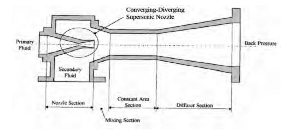
Figure 2.2: Cross sectional view of a typical gas ejector
