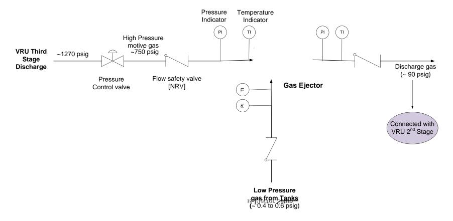
Figure-4.6:Schematic of Gas Ejector Setup
