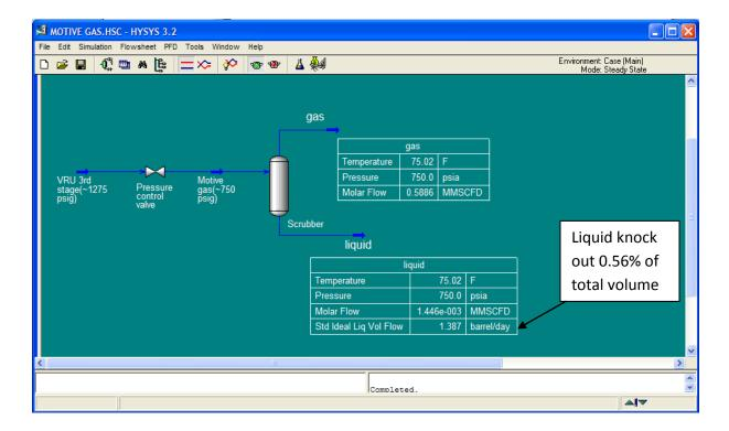
Figure 4.9: Liquid knockout in scrubber due to pressure reduction
