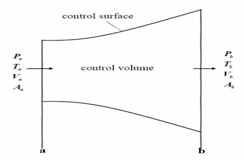
Figure 4.3: Control volume for 1-D flow through converging-diverging nozzle
