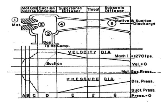
Figure 2.4: Velocity-Pressure changes in a Gas Ejector
