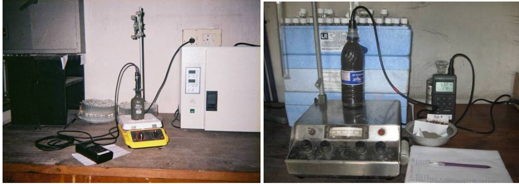
Fig 4.6: Laboratory setup for ex-situ SOD measurement
