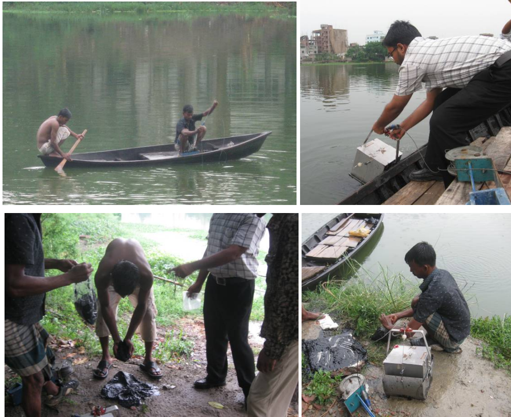
Figure 4.5: Sediment sample collection with a sediment sampler from Gulshan Lake
