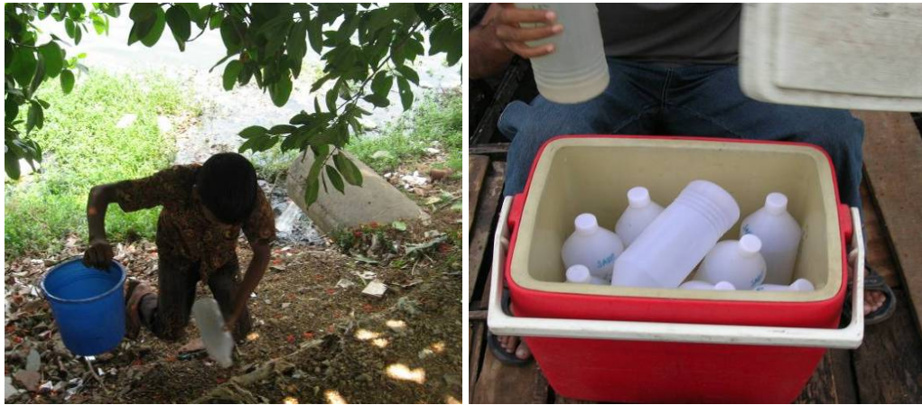
Fig 3.11: Collection of outfall sewage sample from outfall O-4 near R#136
