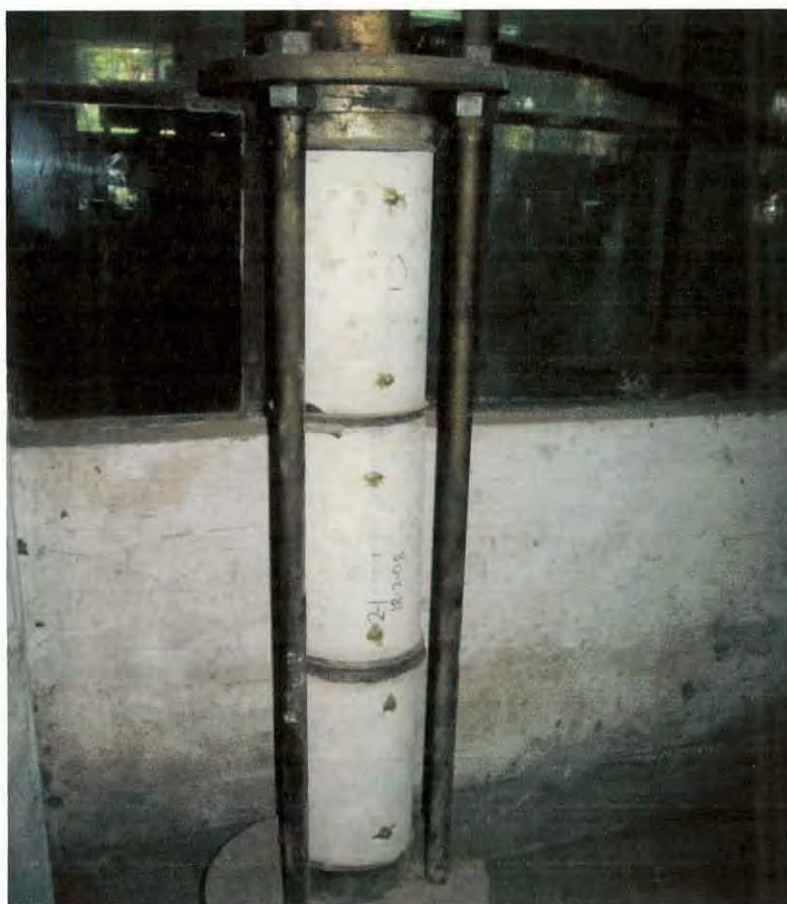
Fig 3.7 Loading Frame with Samples for Creep Testing
