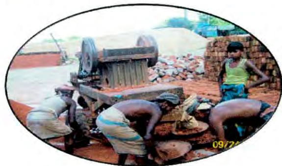
Crushing of bricks by brick crusher
