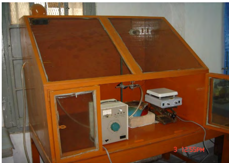
Fig. 3.1 Spray pyrolysis deposition system in Spray Pyrolysis Laboratory, BUET
