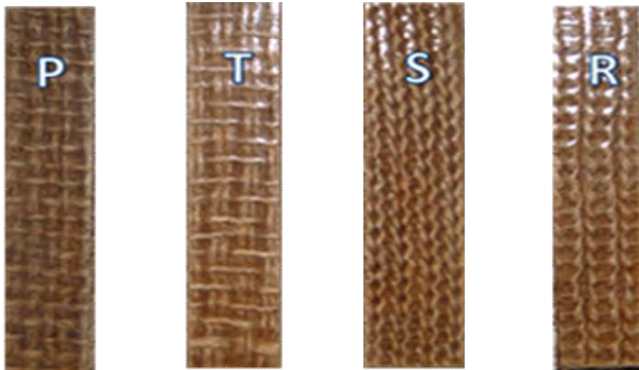
Figure 3.13: Test specimens of PP composites of different fabrics (P- plain, T- twill, S- single jersey, and R- rib) for impact test.
