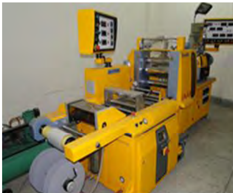
Figure 3.6: Extruder (Lab Tech Engineering Company Ltd. (USA)) machine which was used to produce polypropylene sheet.
