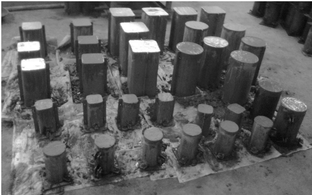
Figure 4.11: Circular and square moulds filled with fresh concrete
