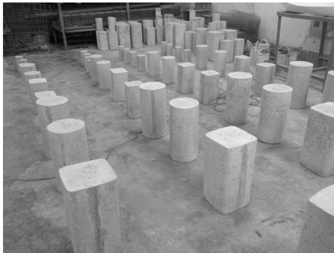
Figure 4.12: Columns after surface preparation. Uneven surfaces are made even using grinding machine.
