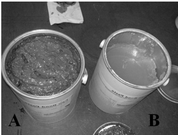
Figure 2.6: Epoxy resins used to bond FRP with concretes (part A and B).
