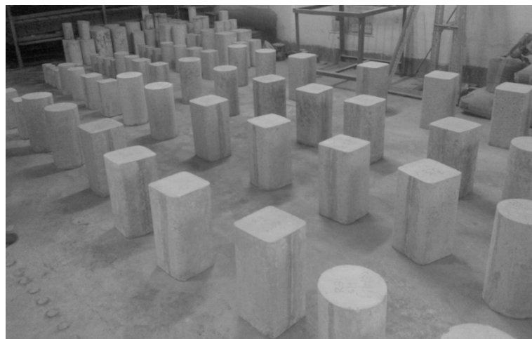
Figure 2.8: Columns prepared for primer coating and FRP wrapping
