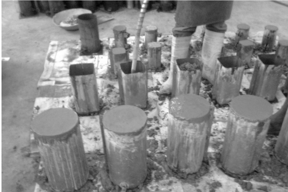
Figure 4.10: concrete compacted in layers using mechanical vibrator
