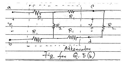
Find  $R_1$  and  $R_2$  so that  $R_{ab} = R_L = 600 \Omega$
