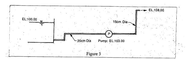
Assume the head loss in the pipe as two times the velocity head at the suction side and 10 times the velocity head in the delivery pipe. Draw a neat sketch showing the hydraulic grade line and the energy line.
