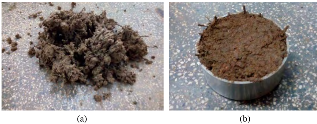
Fig. 3.6 (a) soil and root mixture and (b) specimen in a ring
