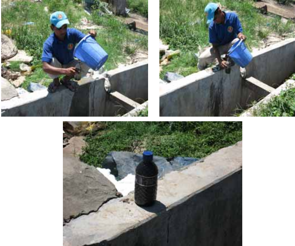
Figure 3.3: Method of leachate collection from semiaerobic system and Boundary system of Matuail Landfill site
