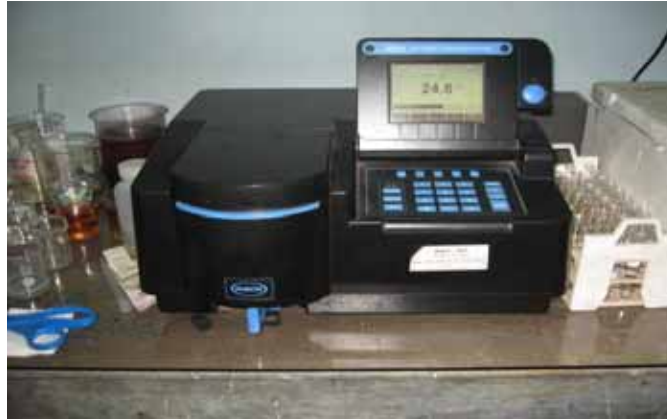
Portable Spectrophotometer (MODEL- HACH, DR4000U).
