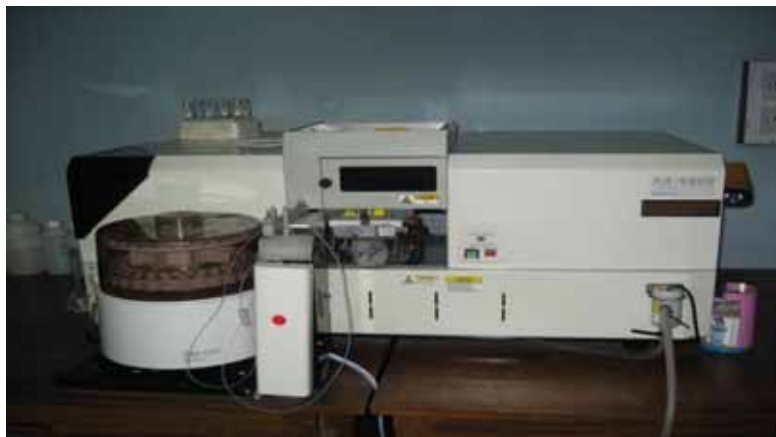
Atomic Absorption (flame) Spectrophotometer (Shimadzu Model No. AA680).
