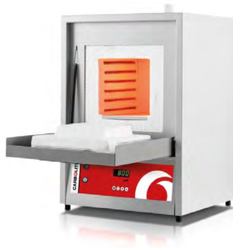
Figure 3.4: Furnace used for annealing xerogel sample
