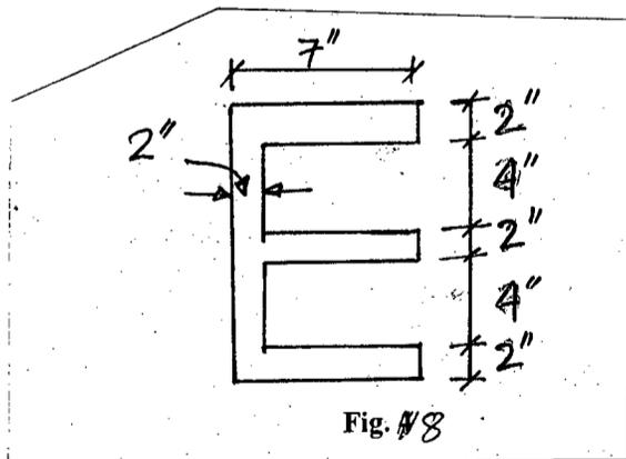
7. (a) Locate the centroid of the composite section shown in Fig. 9. (15)
