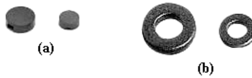
Fig. 3.2 Sample (a) disk shaped, (b) toroid shaped.
