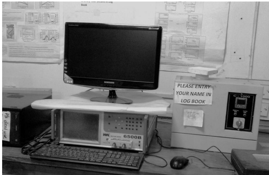
Fig. 3.10 Wayne Kerr impedance analyzer (model no. 6500B).
