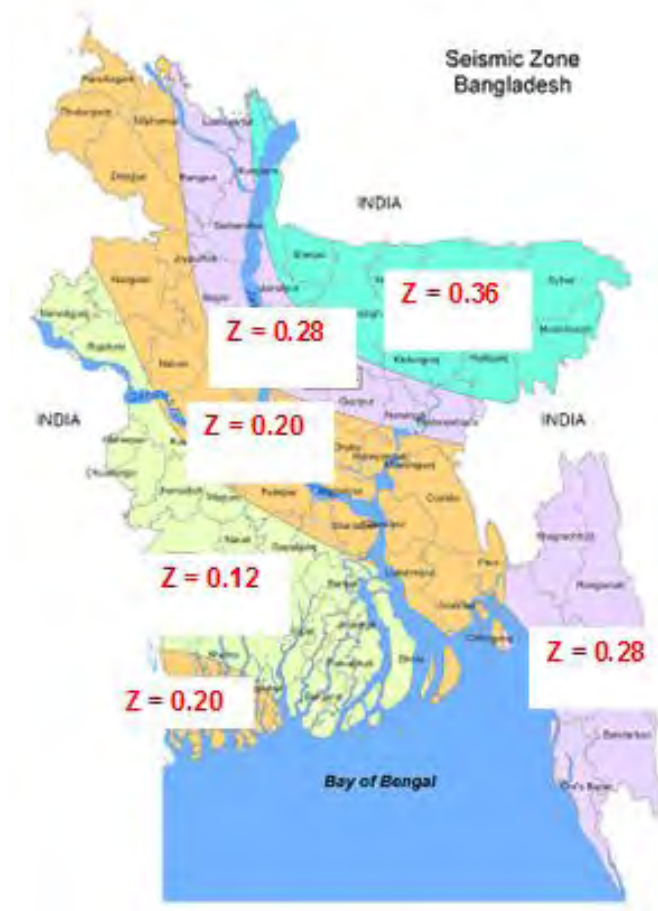
Figure 2.8 Proposed Seismic Zoning Map for Bangladesh based on Maximum Considered Earthquake (Al-Hussaini et al. 2012)
