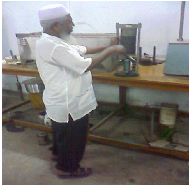
Figure 4.7: Specimen is being removed after Compaction
