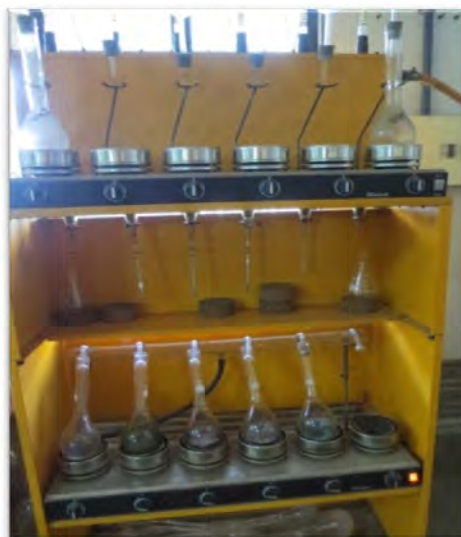
Figure 3 - 4: Kjeldahl Digestion Apparatus
