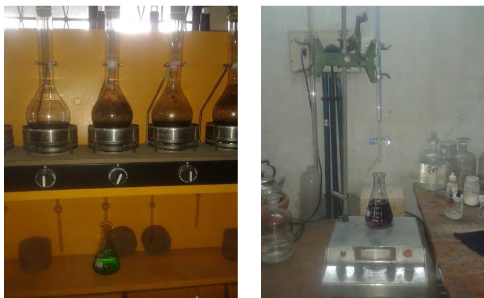
Figure 3 - 5: Collection of distillates in conical flask from Kjeldahl Apparatus (Left) and determination of Total Kjeldahl Nitrogen from the distillates by titrimetric method (Right).
