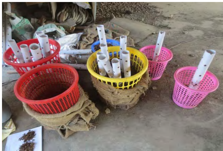
Figure 3 - 3: Composting unit with Jute bag wrapped around to restrict loss of finer particles throughout the composting period
