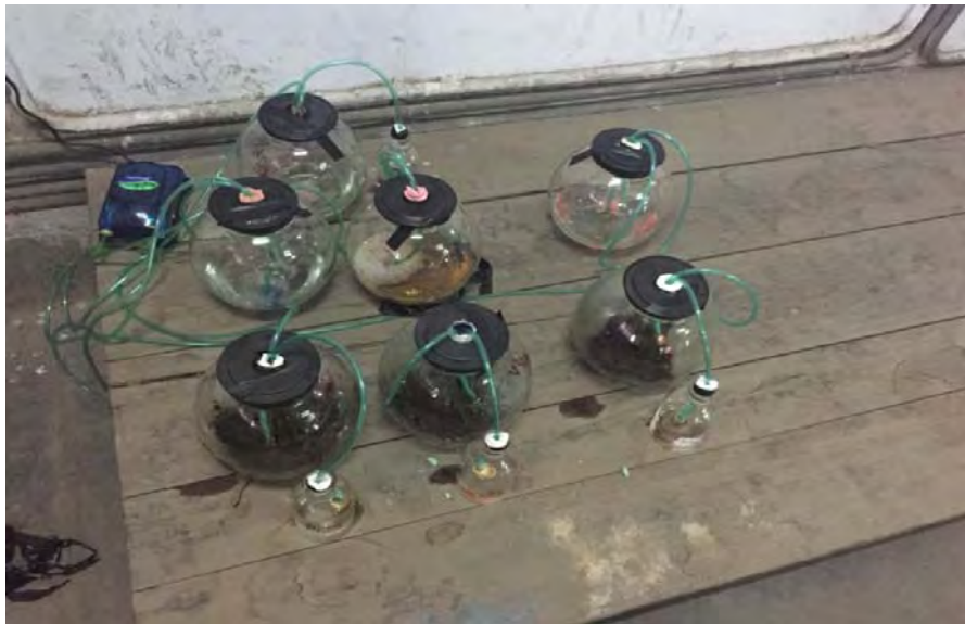
Figure 3 - 7: CO 2 evolution test by using air tight unit to capture the evolved CO 2 gas in NaOH base solution.
