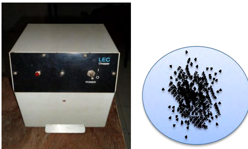
Fig. 4.2.6: Photographs of chopper machine and chopped extrudates.
