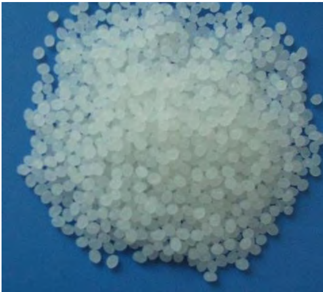
Fig.4.1.1: A photograph of PLA granules
