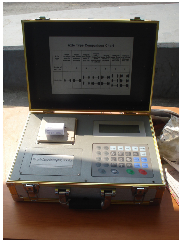
Fig 5.25: Portable Axle Load Measure Unit in Gomoti Toll Plaza
