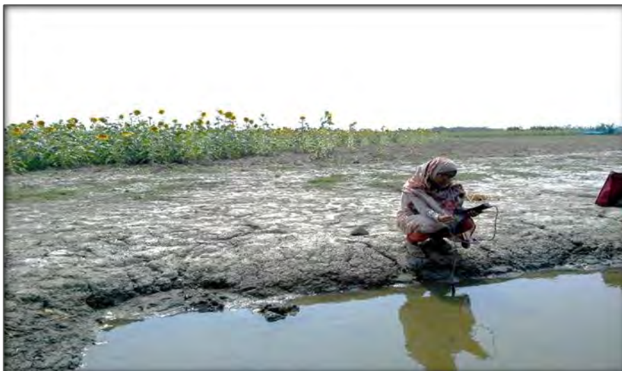
Photo 3.5: Measurement of the EC of water (OFR)
