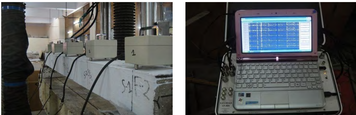
Figure 3.5: sensor and Data Acquisition System of MT
