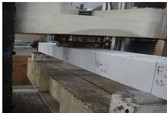
Figure 3.4: Load Application Mechanism in RC Beam
