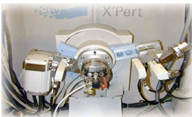
Fig.4.2 PHILIPS PW 3040 X'pert PRO X-ray diffractometer used for XRD.
