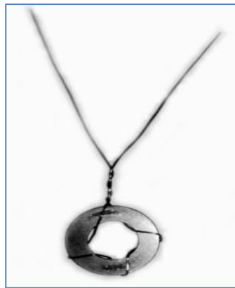
Fig.4.6 winding of four turns on the sample core.
