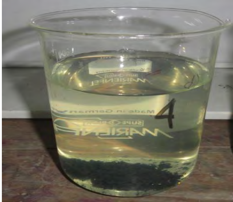
Figure 3.6 Typical scenario of the wastewater after settling down for 30 minutes
