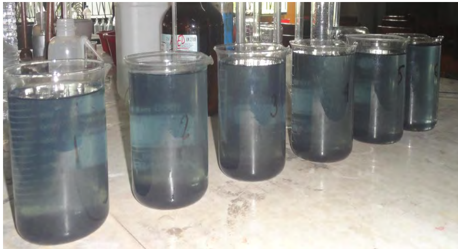
Figure 3.2 Typical raw wastewater sample from denim washing plant
