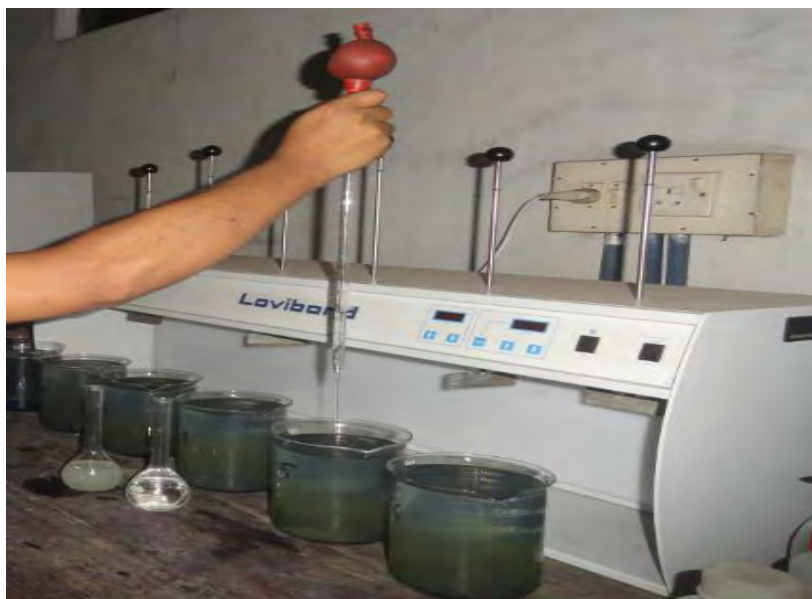
Figure 3.4 Dosing of individual chemicals into the raw wastewater
