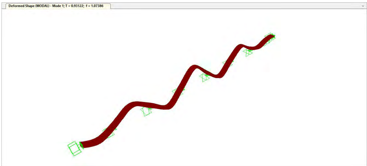
Figure 4.71: 3D View of Mode Shape 1 for First Model (T=0.93)
