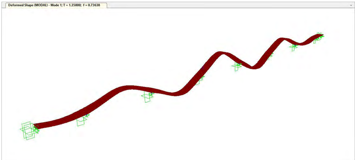
Figure 4.83: 3D View of Mode Shape 1 for Second Model (T=1.36)
