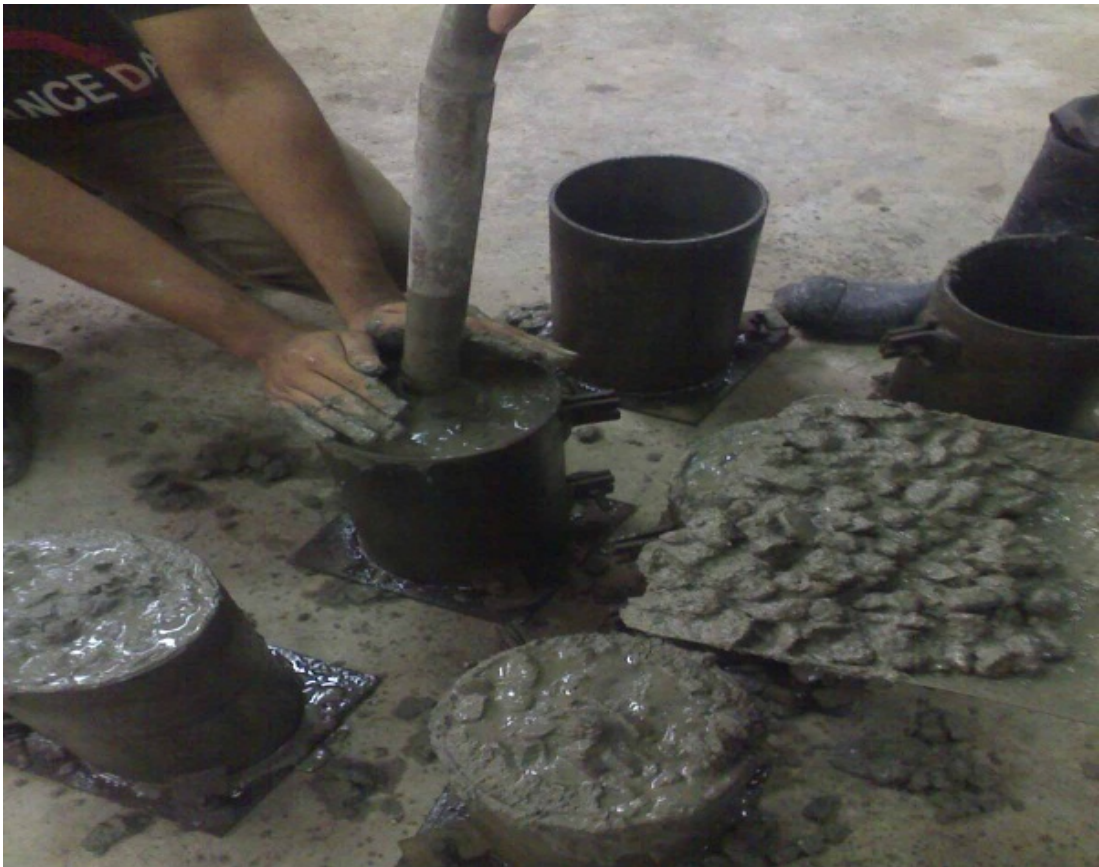
Fig.3.8: Concrete compaction & vibration
