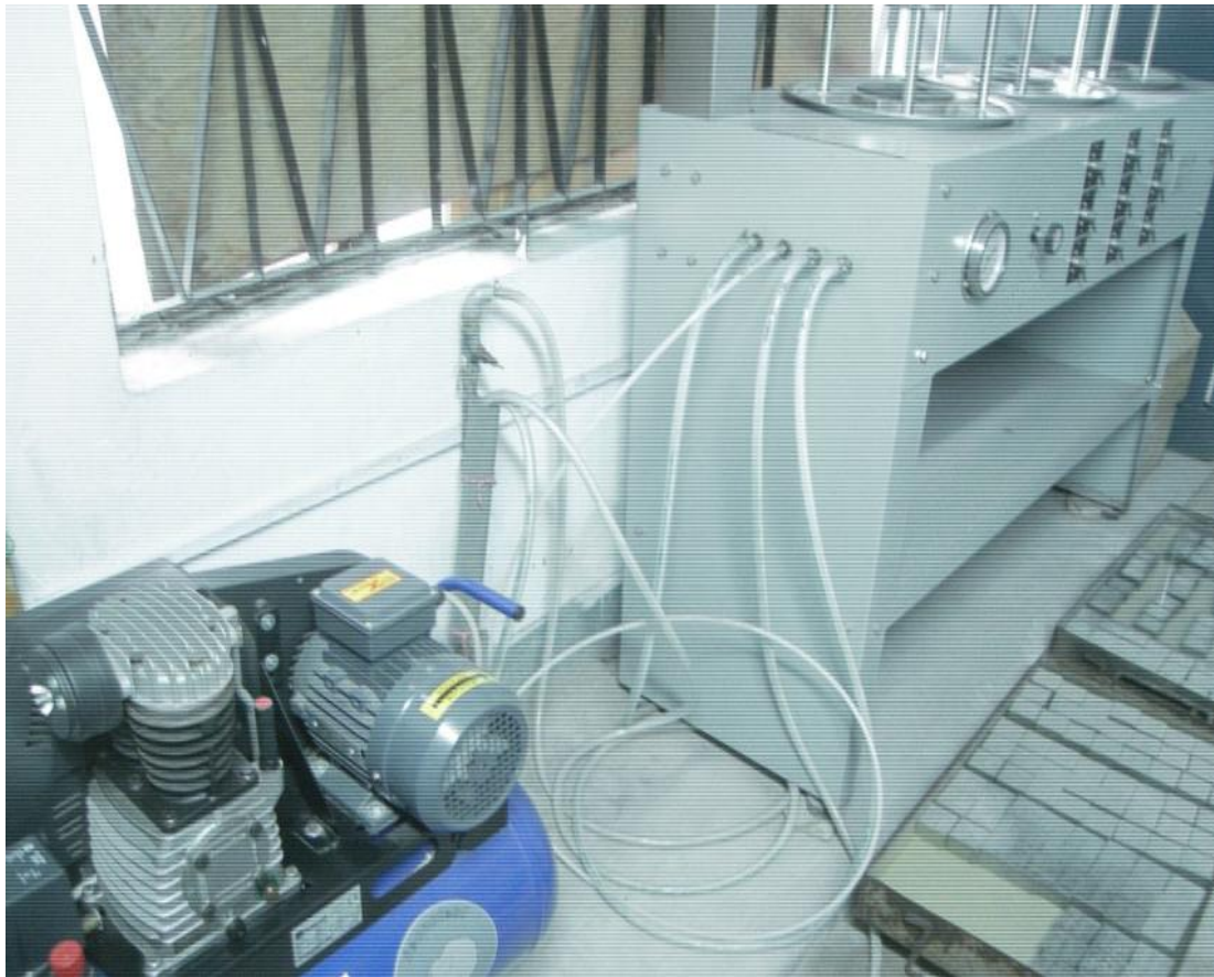
Fig 3.19: Connection between air compressor & specimen testing machine
