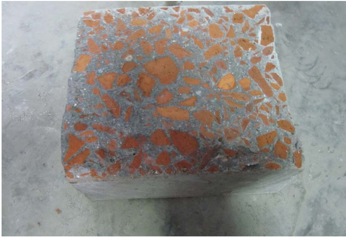
Fig-A1: Wet surface (brick aggregate concrete)
