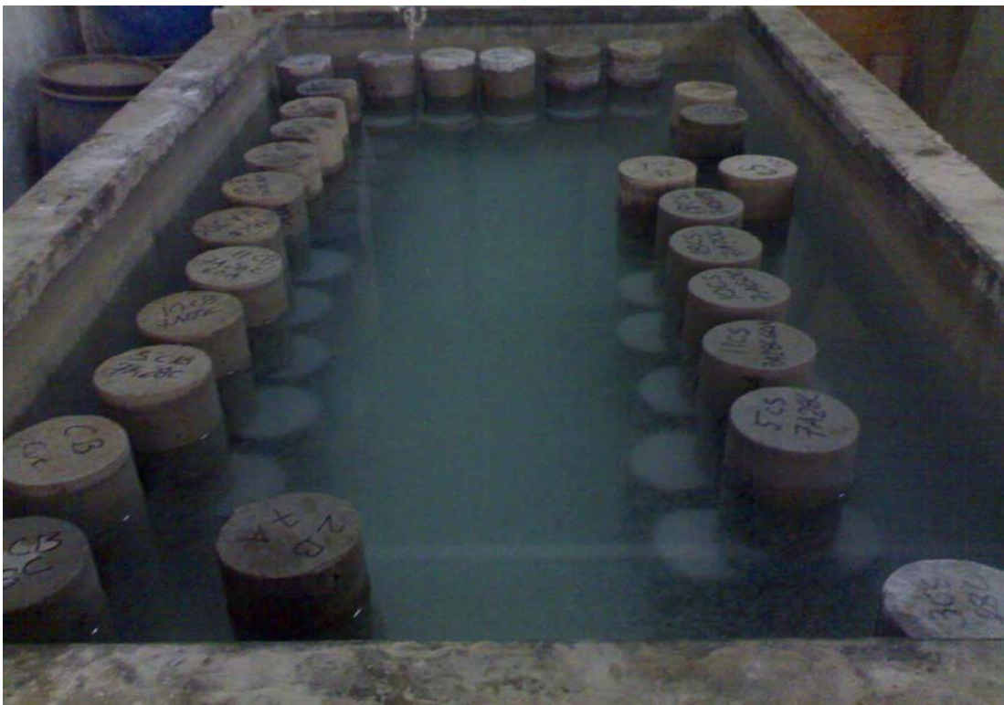
Fig.3.9: Curing of cylinders and cube
