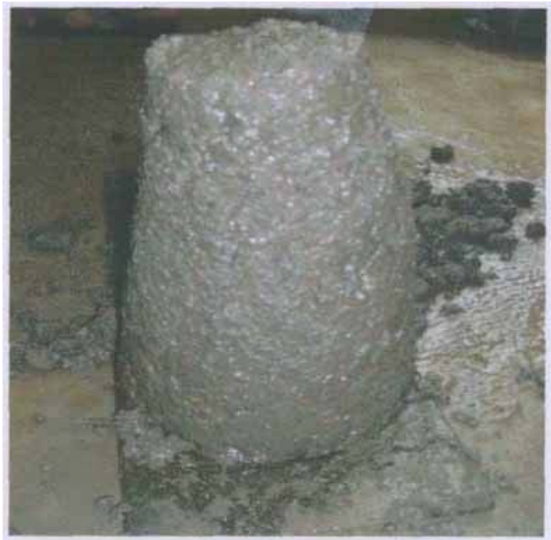
Fig.3.12: Slump test of concrete.
