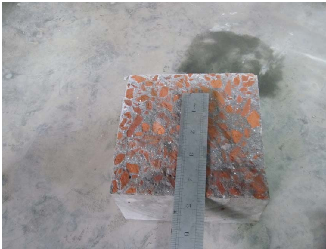
Fig 3.21: Depth of penetration of water (brick aggregate concrete)
