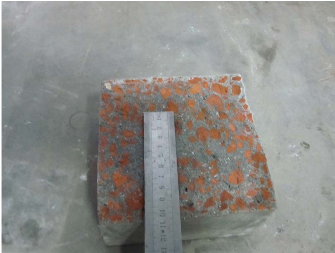
Fig 3.21: Depth of penetration of water (brick aggregate concrete)
