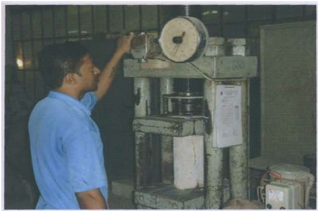
Fig. 3.15: Compressive strength test
