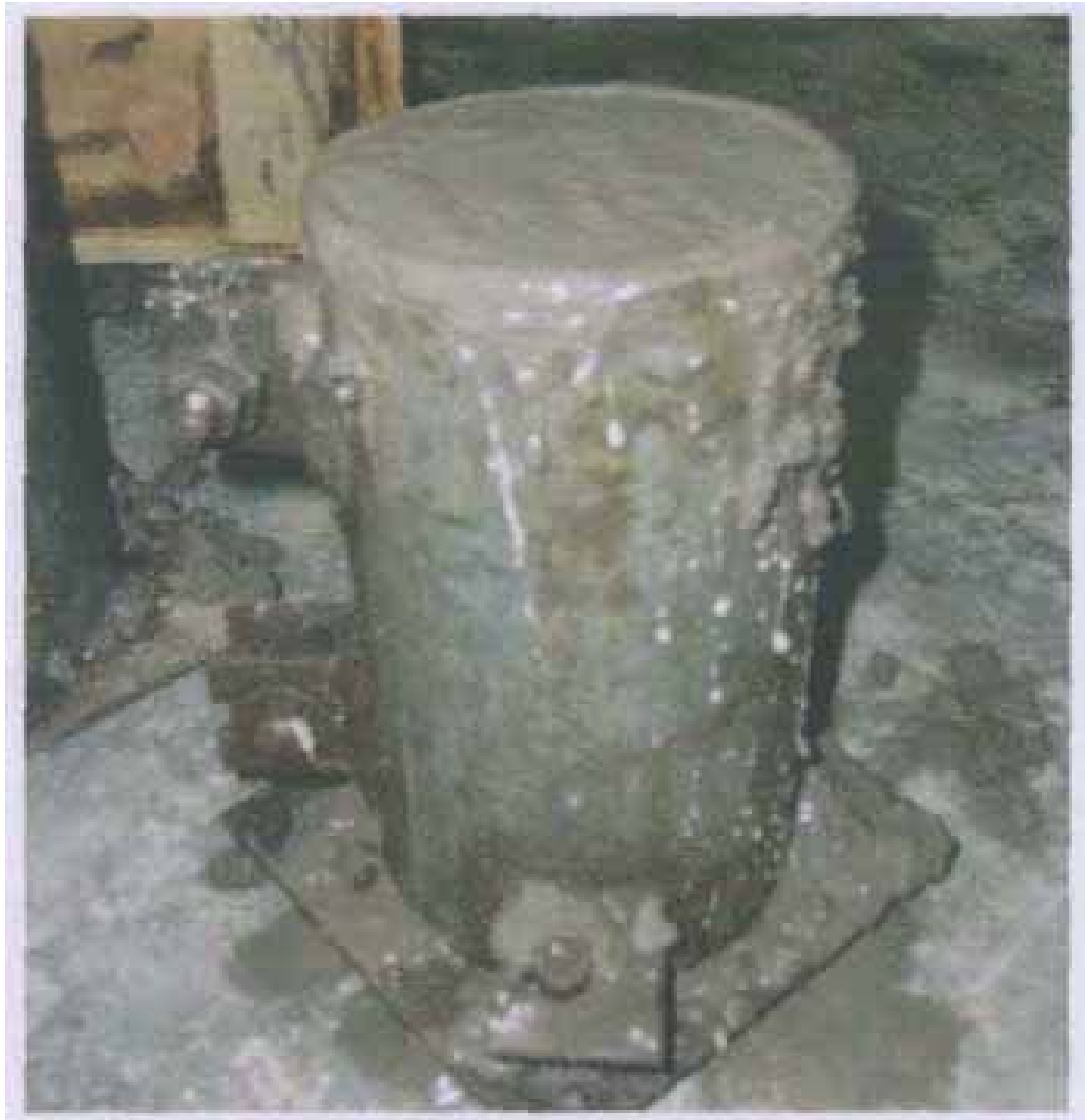
Fig.3.14: Concrete pouring in cylinder
