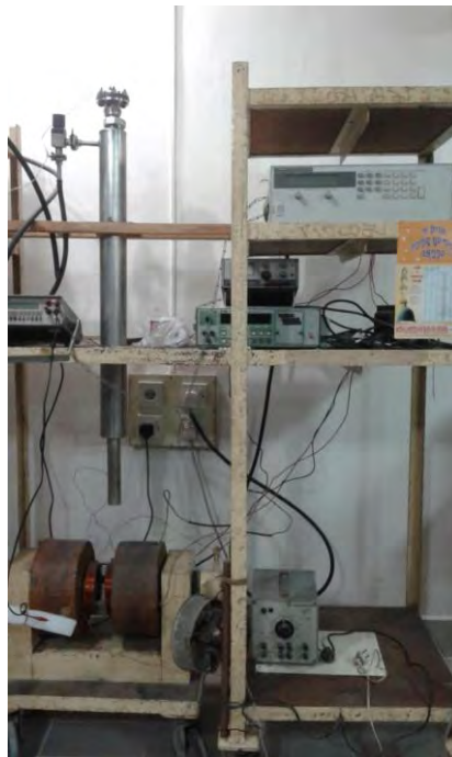
Fig. 3.8 Experimental set up for the measurement of magnetolectric coefficient.
