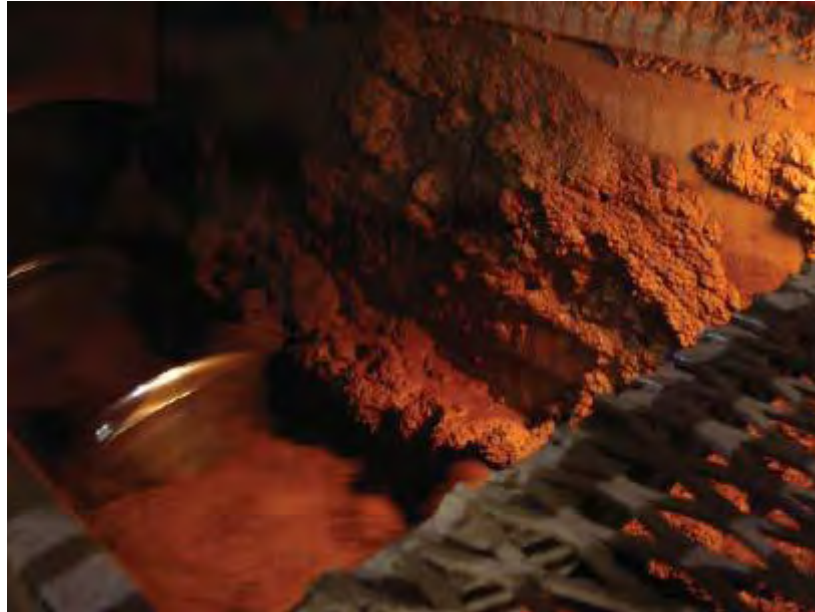
Figure 2.7. Clay is thoroughly mixed with water in pug mill extrusion. Source: ( Brick Industry Association 2006 )
