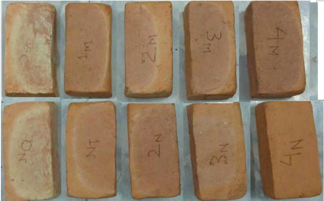
Figure 3.6. Bricks after firing at muffle furnace (N.B: In Figure 3.6; 0, 1, 2, 3, 4 indicates 0%, 10%, 30% and 40% sludge amended bricks and M & N indicates firing temperature of 1000°C and 950°C, respectively.)
