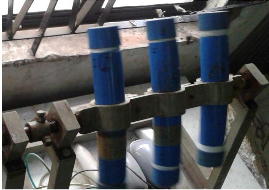
Figure 3.10. An arrangement for carrying TCLP test according to USEPA 1311
