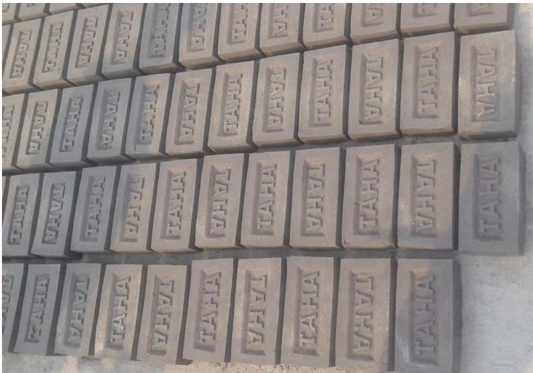
Figure 3.7. Brick prepared in the kiln (Field condition)
