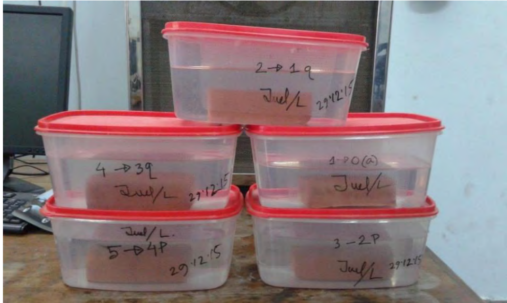
Figure 3.11. An arrangement of the leaching test (according to NEN 7345) being carried out in the laboratory with sludge-amended bricks.
