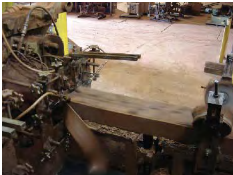
Figure 2.8. Clay is extruded through a die and trimmed to specified dimension before firing. Source: ( Brick Industry Association 2006 )
