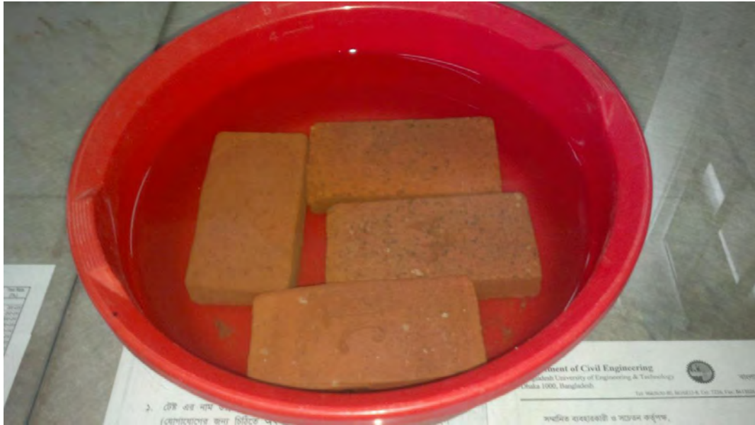
Figure 3. 9. An arrangement of conducting water absorption test.
