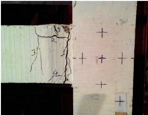
Fig. 5.5: Appearance of First Flexural Crack
