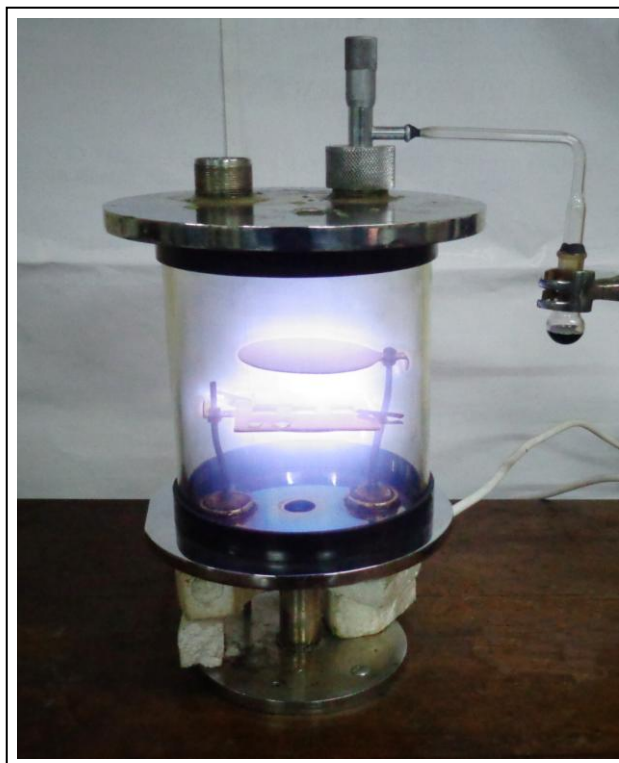
Fig. 3.5: Glow discharge plasma during deposition
