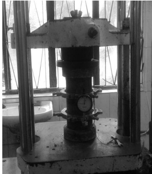
Figure 4.5: Test setup for Modulus of Elasticity
