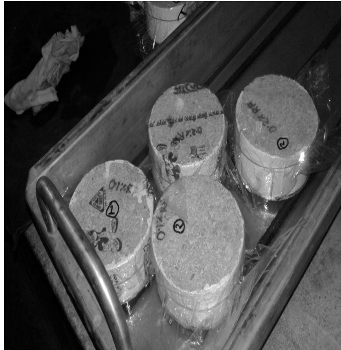
Figure 4.6: Test setup for rate of water absorption (sorptivity)
