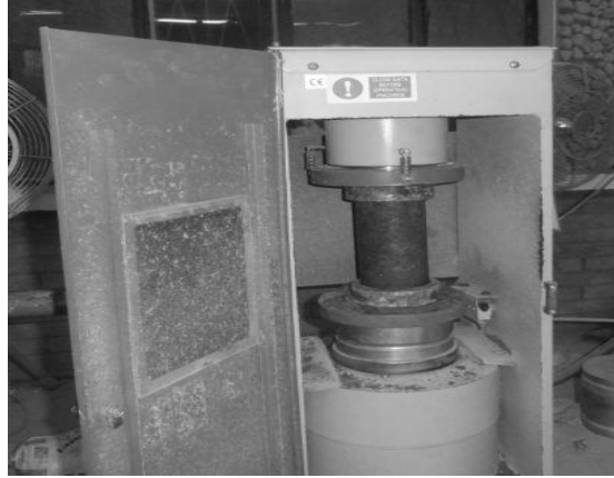
Figure 4.3: Test setup for compression test of cylinders
