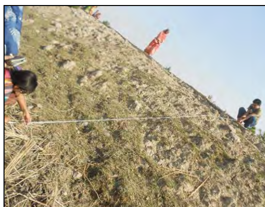
Photo B6: Measurement of Polder height during field visit.
