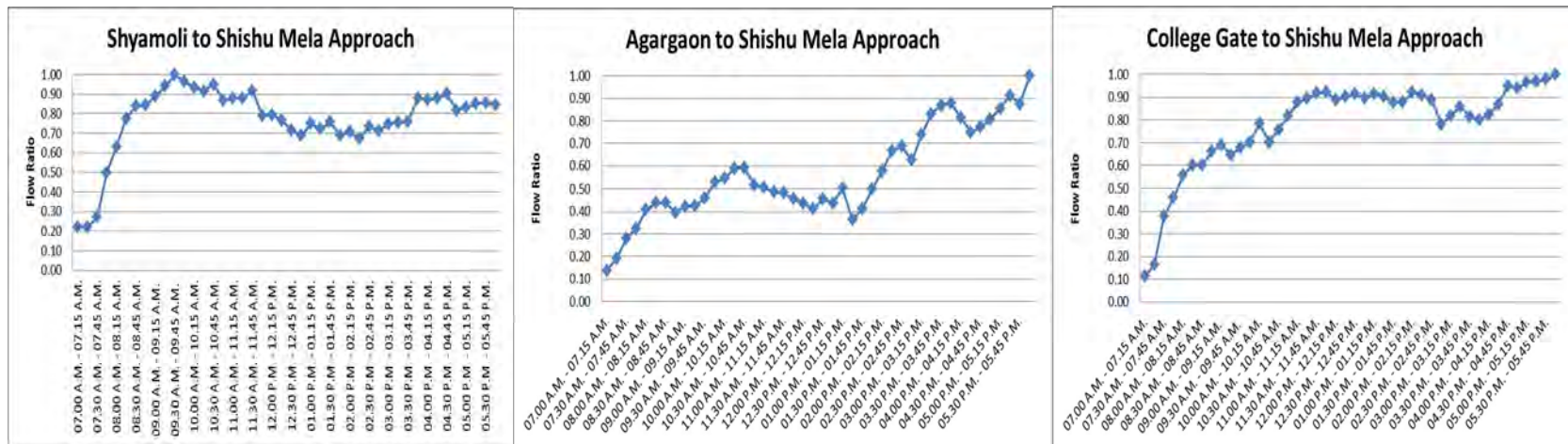
Figure 1.2.8: a) Flow Ratio of Shyamoli to Shishu Mela Approach; b) Flow Ratio of Agargaon to Shishu Mela Approach; c) Flow Ratio of College Gate to Shishu Mela Approach.
