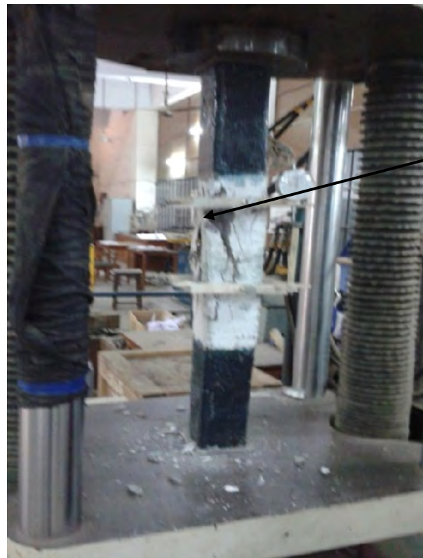
Figure 4.17 Failure modes of column SCN4E
