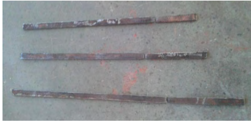
Figure 4.6 Structural steel plate samples for tension test
