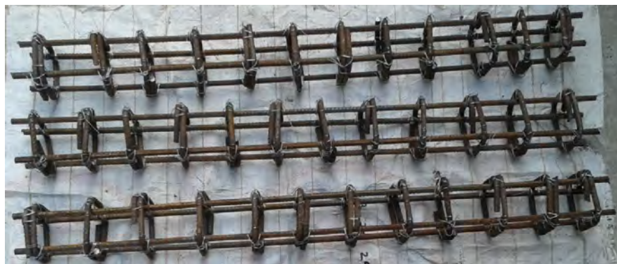
Figure 4.2 Reinforcements for FEC columns
