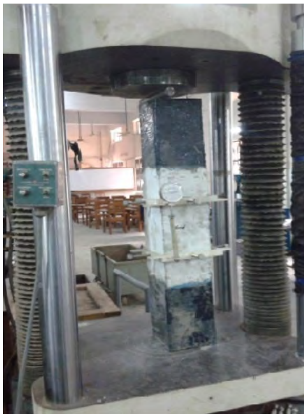
Figure 4.11 Test set up for eccentric axial load in laboratory
