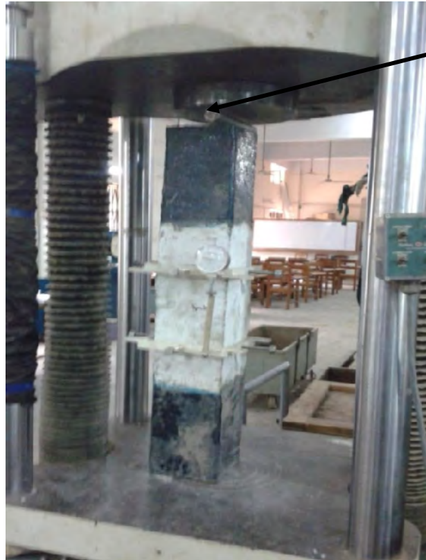
Figure 4.18 Failure modes of column SCH6E
