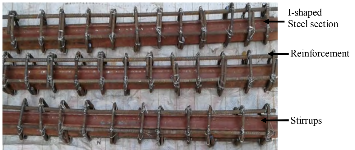
Figure 4.4 Structural steel with reinforcement in FEC columns
