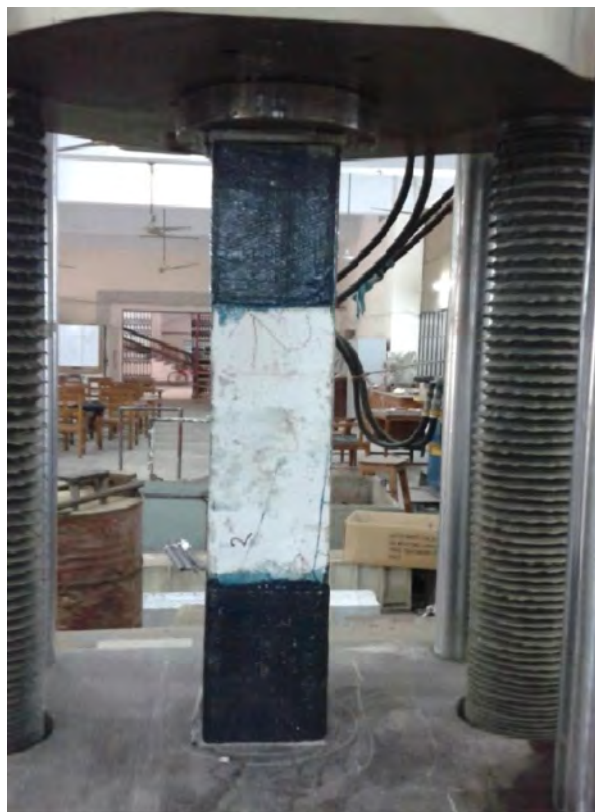
Figure 4.10 Test set up for concentric axial load in laboratory
