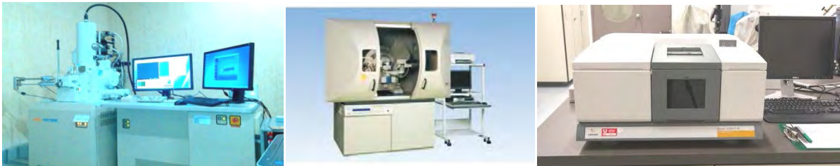
Figure 2.2: Images of EDX integrated SEM, XRD, FTIR instruments(from left)
