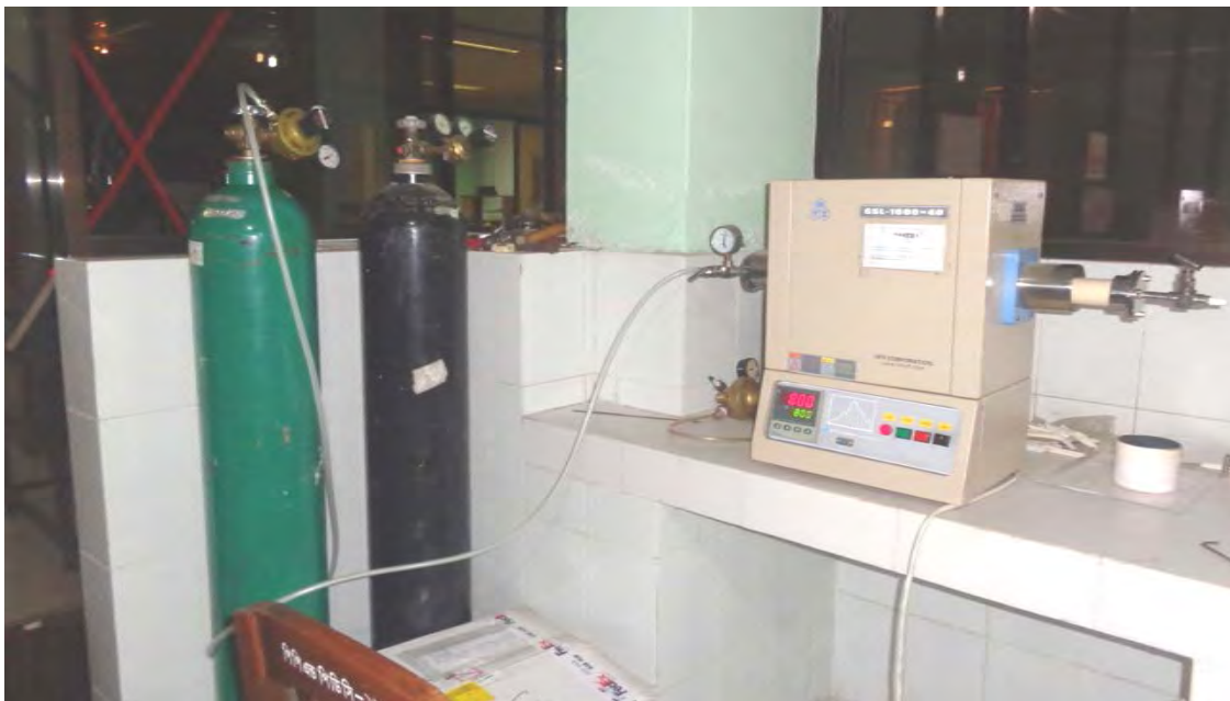
Figure 2.1: Argon gas controlled high temperature furnace
