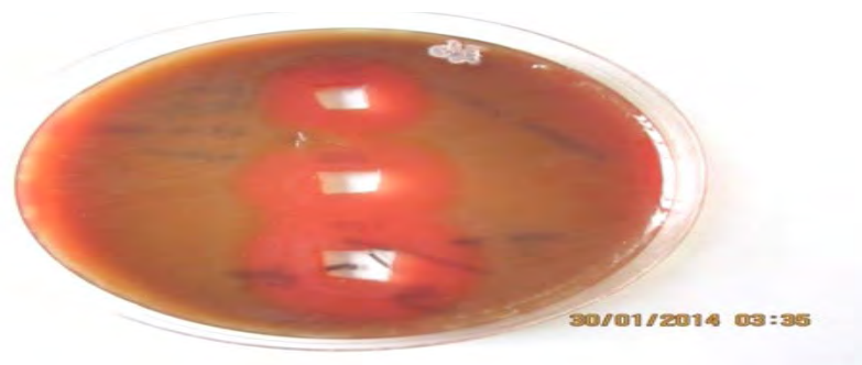
Figure 3.36: Image of zone inhibition for Streptococcus pneumoniae by the pure Mn 3 O 4 nanoparticles
