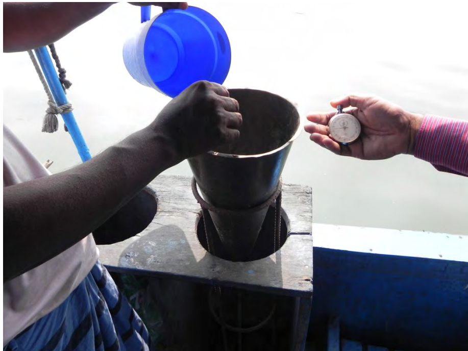
Fig. 4.7: Sample being transferred from the container to the measurement tube using a funnel
