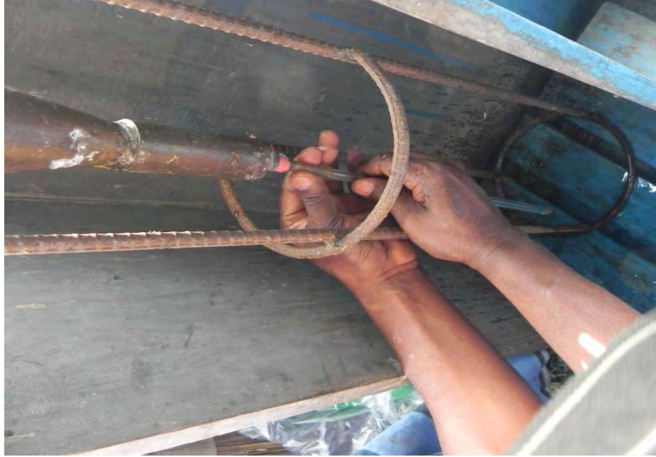
Fig. 4.8: Measurement tubes being separated after collection of sample
