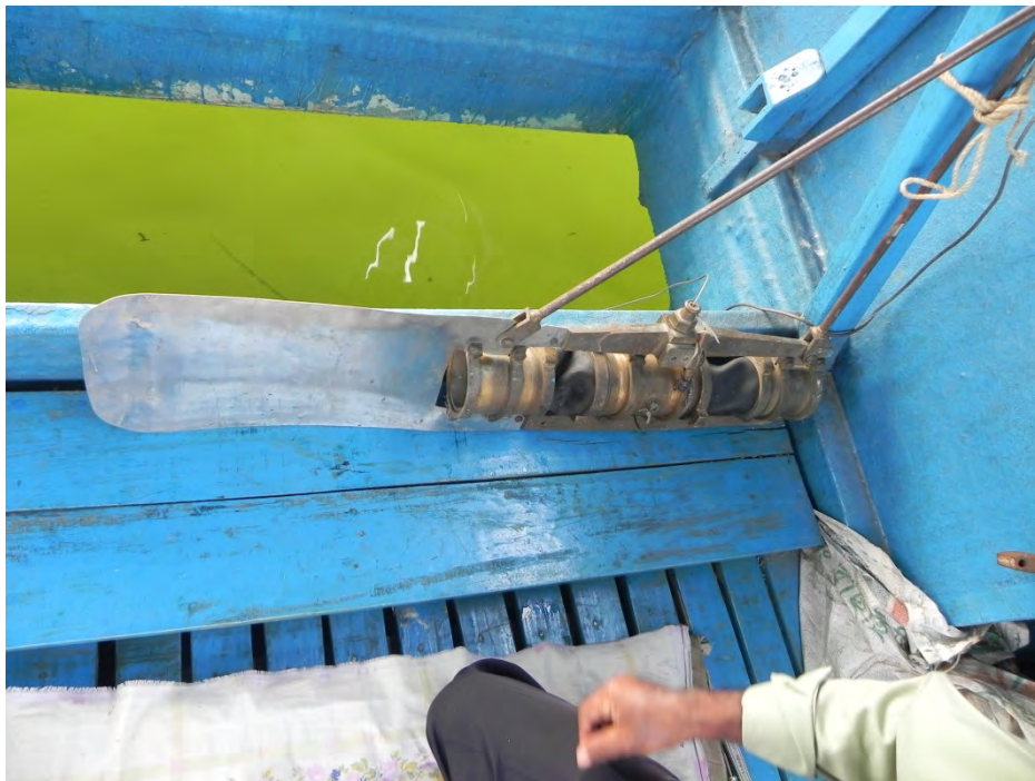
Fig. 4.3: Sediment gauging equipment being prepared for sample collection
