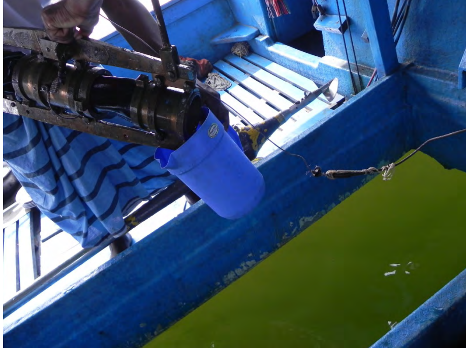
Fig. 4.6: Water sample being transferred to another container from sediment sampling equipment
