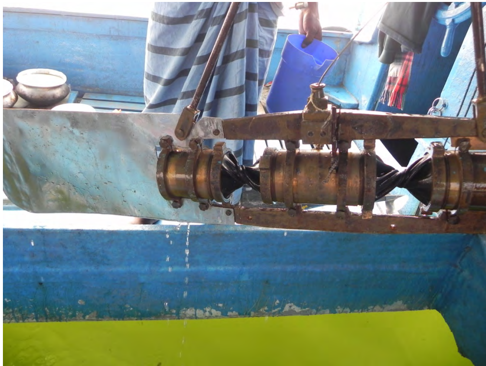
Fig. 4.5: Sediment sampling equipment being lifted up after water sample collection
