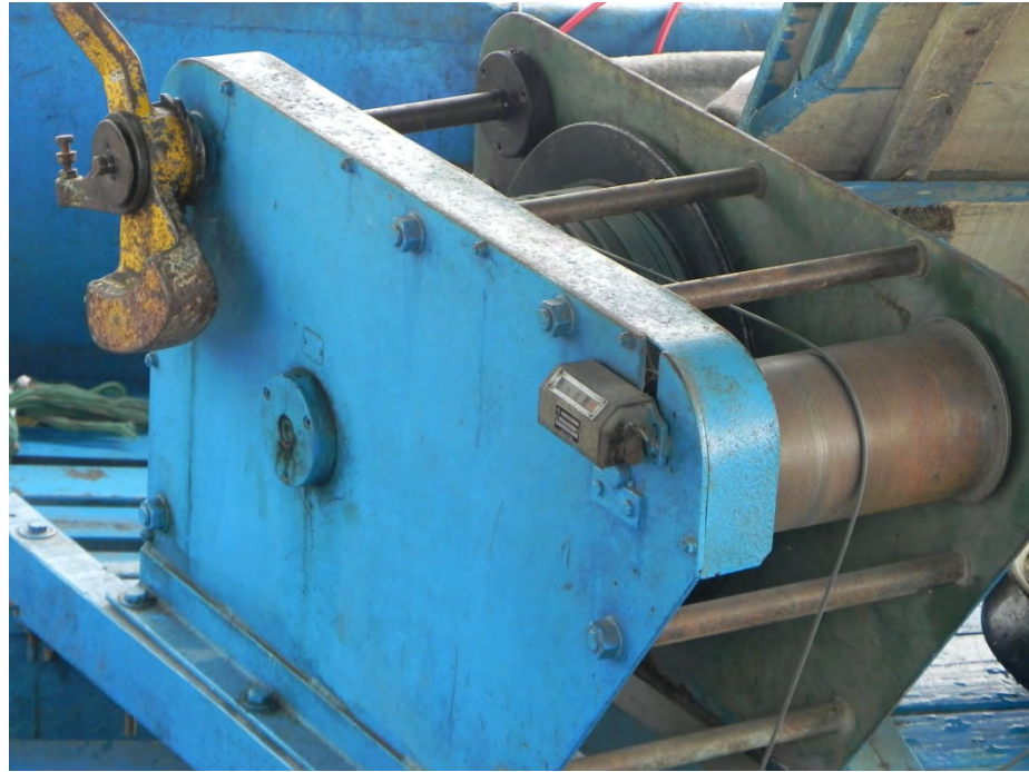
Fig. 4.2: An automatic pulley system used to lift and submerge gauging equipment
