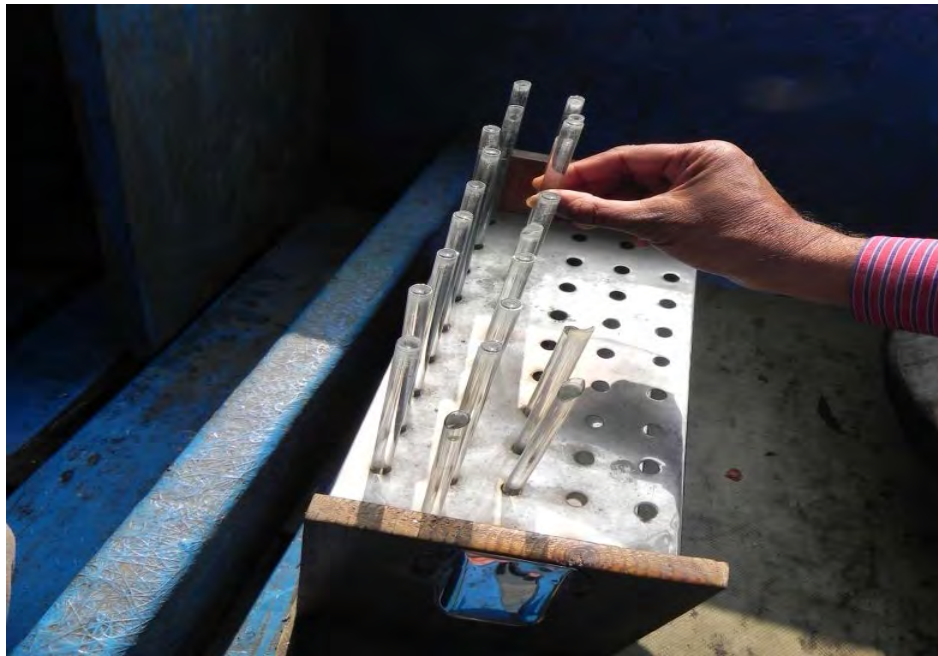
Fig. 4.9: Samples in measurement tubes being stored to be transferred to laboratory for testing
