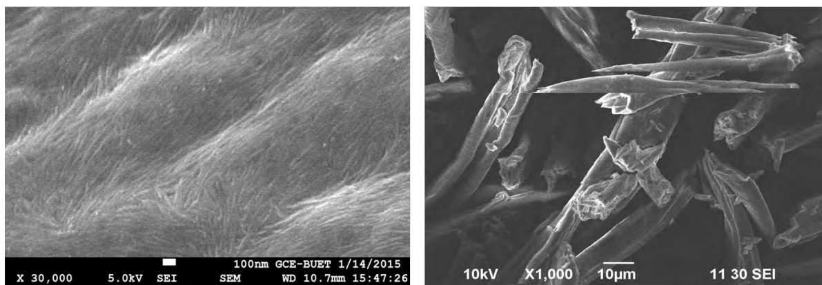
Fig 4.9. (a) FESEM image of NCC and (b) FESEM image of MCC
