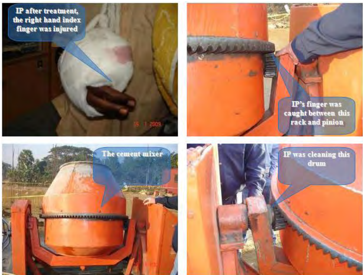
Fig- 8.5 Cement mixing by rotating cement mixer (Personal Injury of JB Plant) [6];
