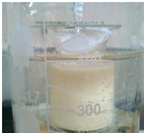
Fig. 3.2: Chemical bath deposition system and films deposition process
