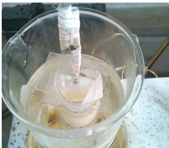
Fig. 3.2: Chemical bath deposition system and films deposition process
