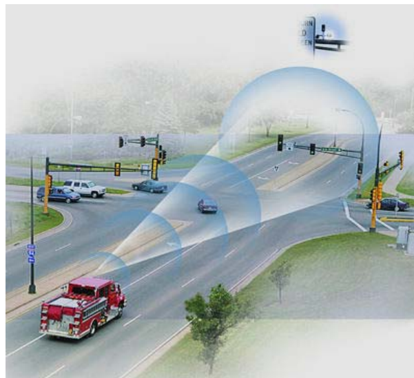
Figure 4.43: Emergency Vehicle Signal Preemption
