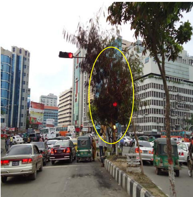
Figure 4.32a) Poor Visibility of Traffic Signal in Hotel Sonargaon
