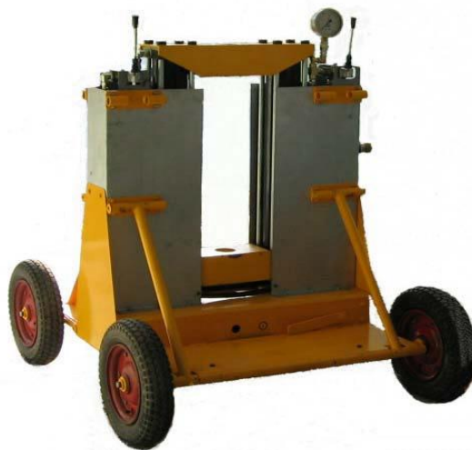
Fig 3.1 : CPT Machine (Ref: Envi 200 kN CPT Pusher / Puller Operating Manual)
