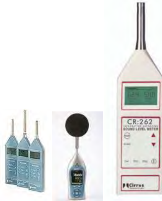
Figure 2.1: Integrating-averaging sound level meters (IEC, 2002).
