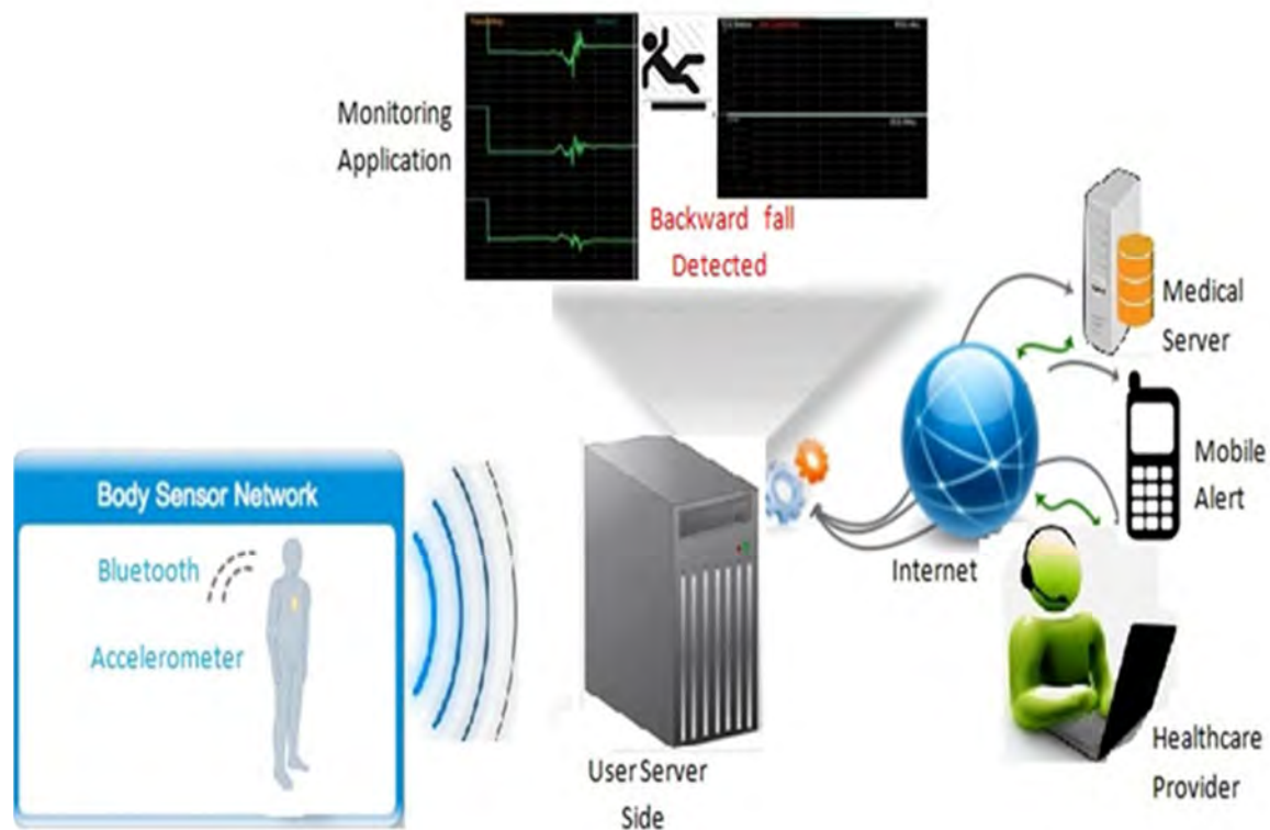
Fig 3.1: Data flow diagram of the direction-sensitive fall detection system
