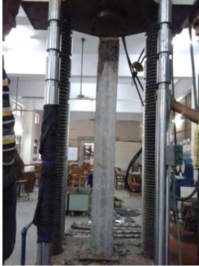
Figure 5.4 Failure mode of un-strengthened RC column under concentric loads
