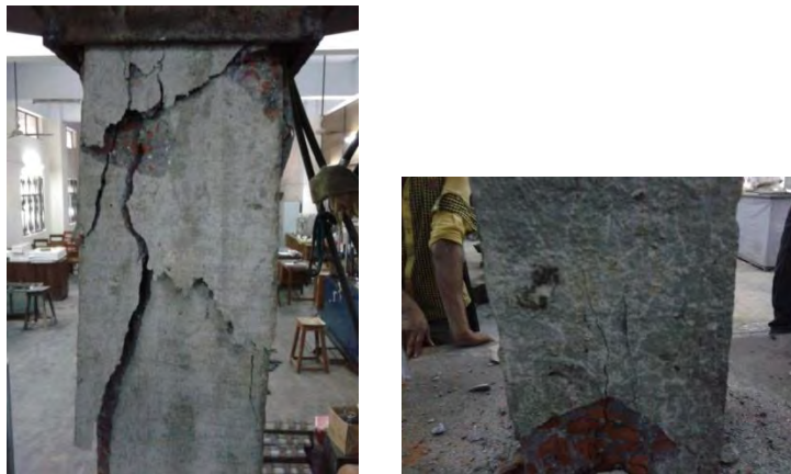
Figure 5.6 (a) Top concrete crushing and (b) Bottom concrete crack of un-strengthened RC column under concentric loads
