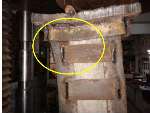
Figure 5.13 Buckling of compression side steel angles at top with an eccentricity of 37.5 mm
