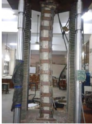
Figure 5.14 Failure mode of strengthened RC column with an eccentricity of 67.5 mm
