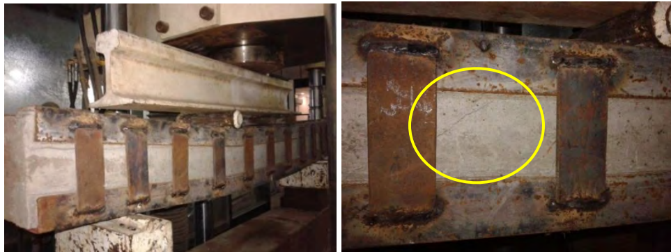
Figure 5.15 Buckling of steel angles and concrete crushing in between strips with eccentricity of 67.5mm
