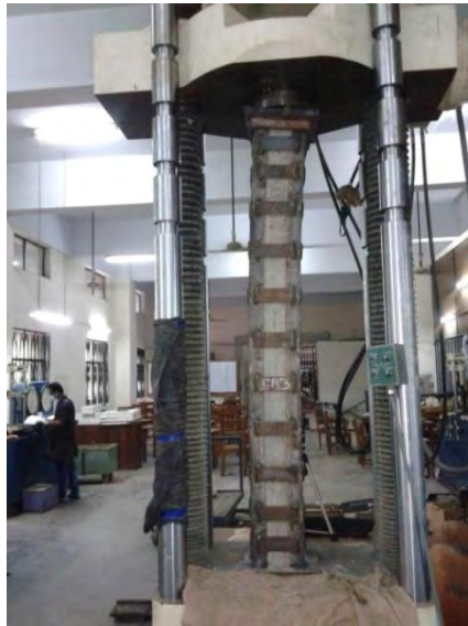
Figure 5.9 Failure mode of strengthened RC column with eccentricity of 15mm
