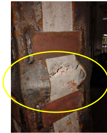
Figure 5.15 Buckling of steel angles and concrete crushing in between strips with eccentricity of 67.5mm
