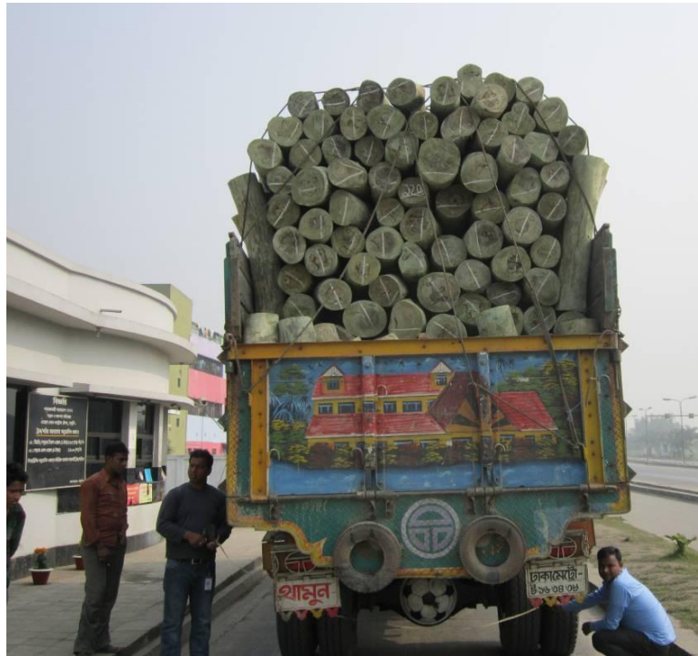
Figure 3.7: Truck Containing Timber Log Weighing 73480 lb (33.4 ton)
