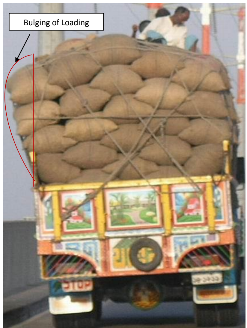
Figure 3.6: Bulging of Loading
