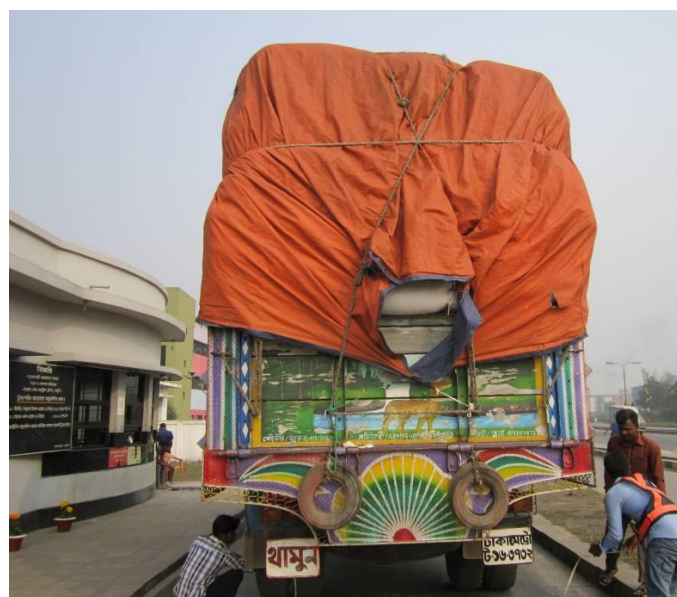
Figure 3.8: Heavy Truck with Overall Height 15.17 ft
