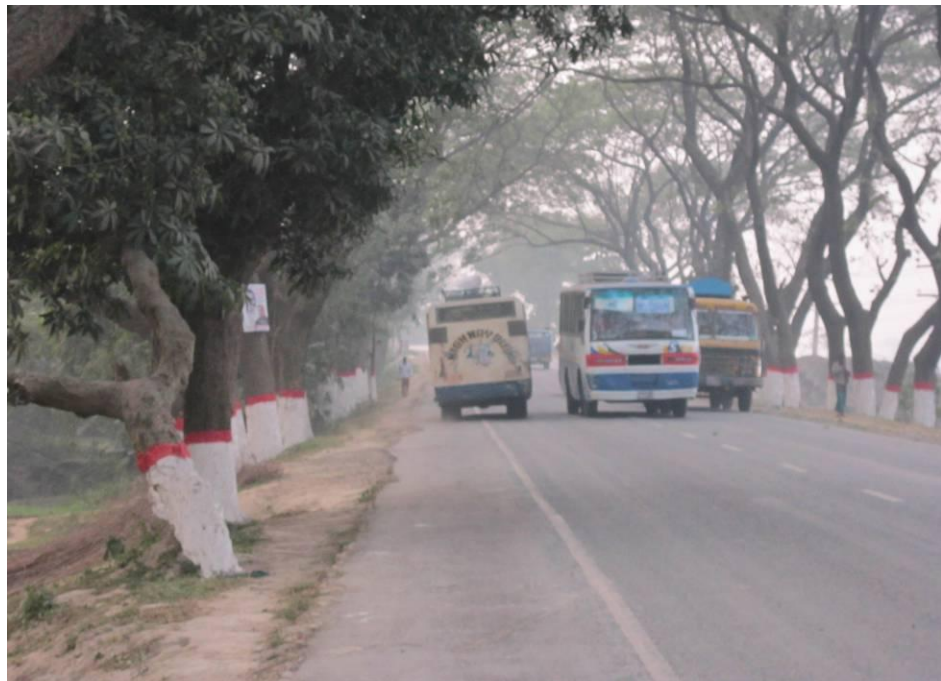
Figure 3.5: Overtaking of Opposing Vehicle Forces Left Lane Bus to Encroach on to Shoulder
