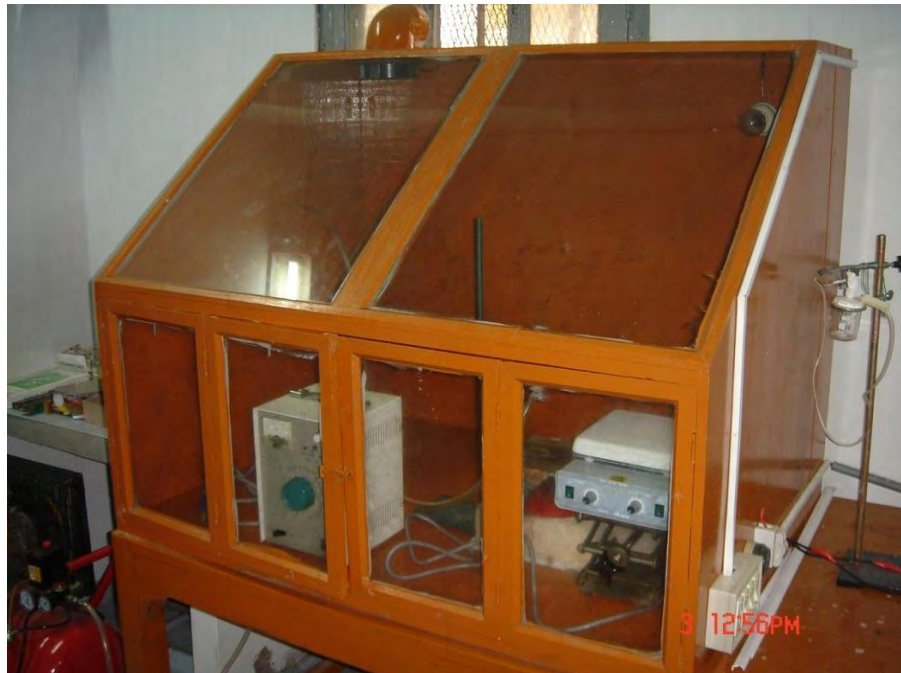
Figure 4.4: Experimental set up of Spray Pyrolysis unit at the Department of Physics, BUET
