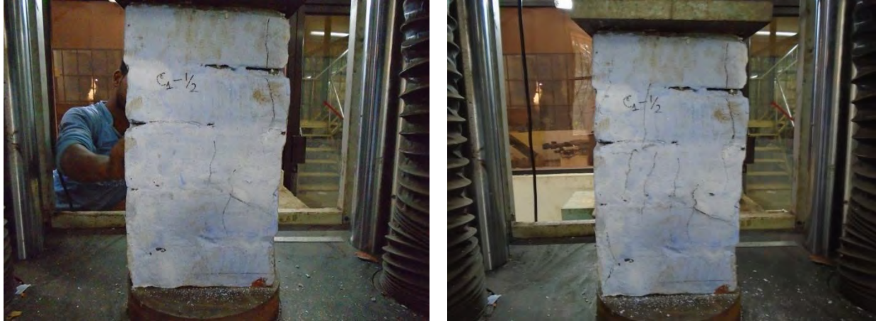
a. Appearance of first crack of prism C1-1/2
