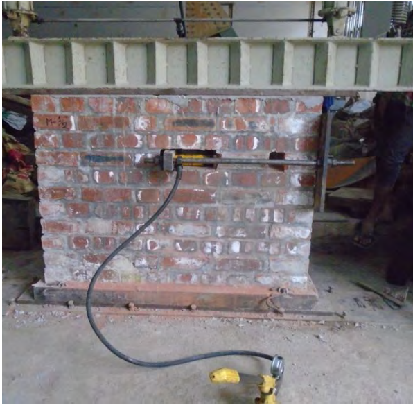
e. Shear test setup of machine made brick wall (M-1/2) with mortar thickness 1/2"
