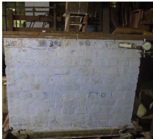
Figure 4.35 2 nd and 3 rd Cracks Patterns of Specimen M1-1/2
