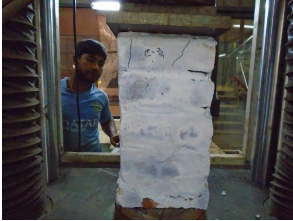
a. Appearance of first crack of prism C-3/4
