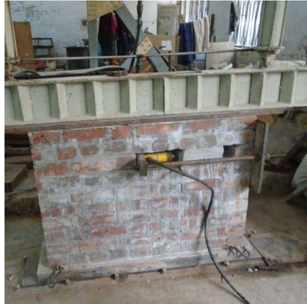
h. Shear test setup of machine made brick wall (M1-3/4) with mortar thickness 3/4"
