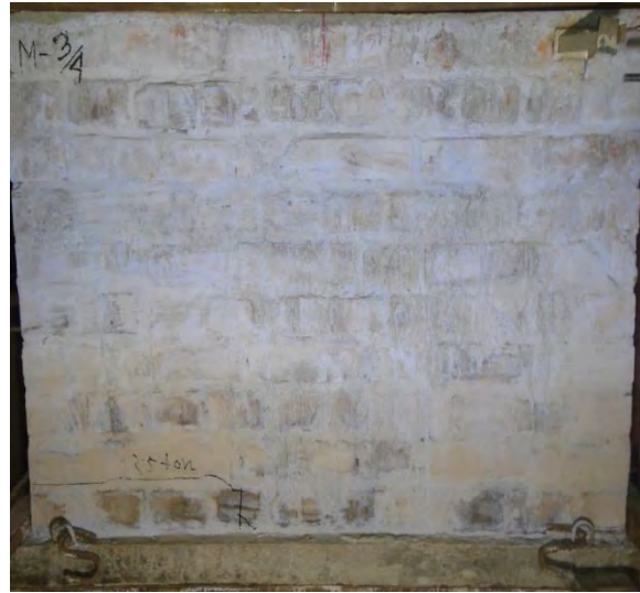
Figure 4.38 2 nd Cracks Patterns of Specimen M-3/4
