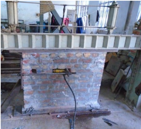
c. Shear test setup of clay burnt brick wall (C-3/4) with mortar thickness 3/4"
