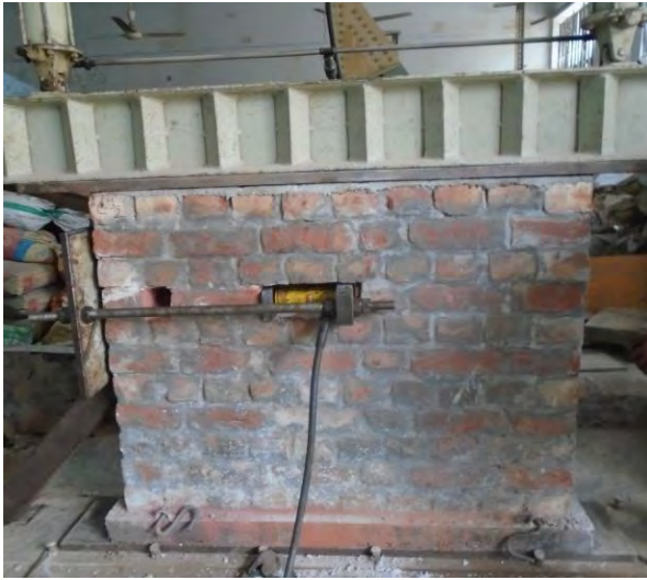
a. Shear test setup of clay burnt brick wall (C-1/2) with mortar thickness 1/2"
