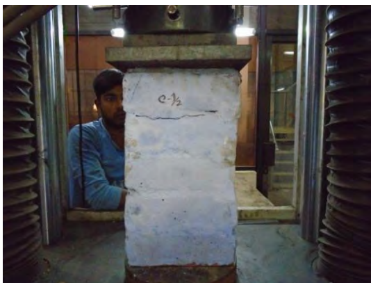
a. Appearance of first crack of prism C-1/2 b. Ultimate crack of prism C-1/2
