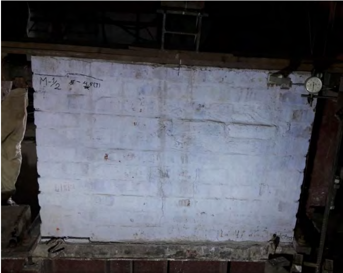
Figure 4.33 Final Crack Pattern of Specimen M-1/2
