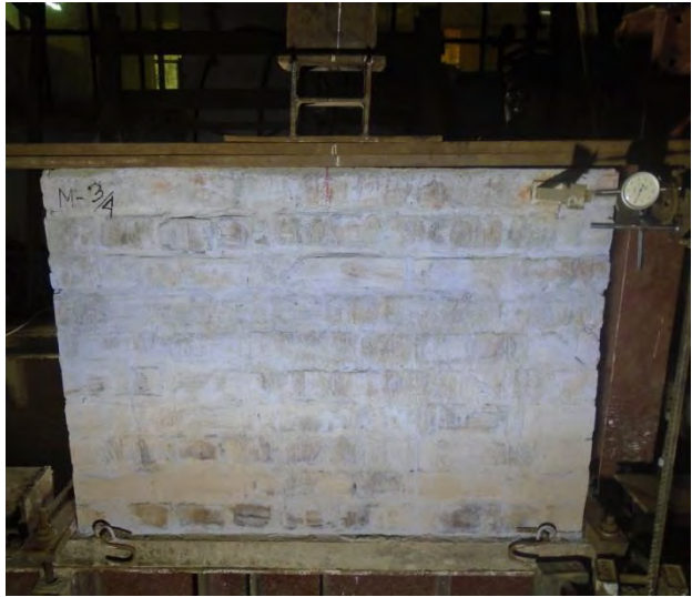
Figure 4.37 Initial Crack (Flexure) Patterns at Specimen M-3/4
