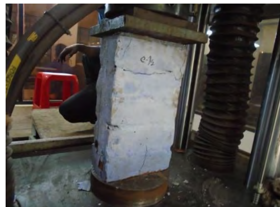
a. Appearance of first crack of prism C-1/2 b. Ultimate crack of prism C-1/2
