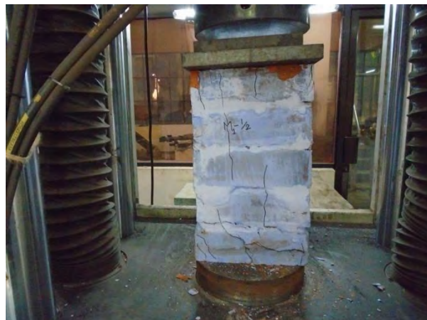
b. Ultimate crack of prism M-1/2
