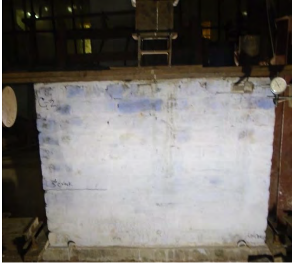
Figure 4.22 3 rd Crack (Shear) Pattern of Specimen C1-1/2
