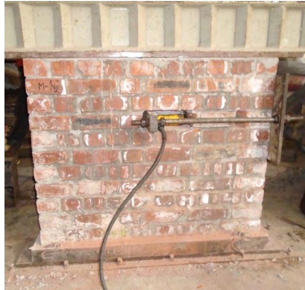
f. Shear test setup of machine made brick wall (M1-1/2) with mortar thickness 1/2"
