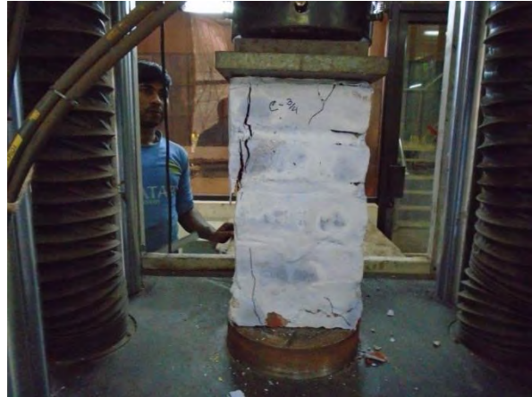
b. Ultimate crack of prism C-3/4
