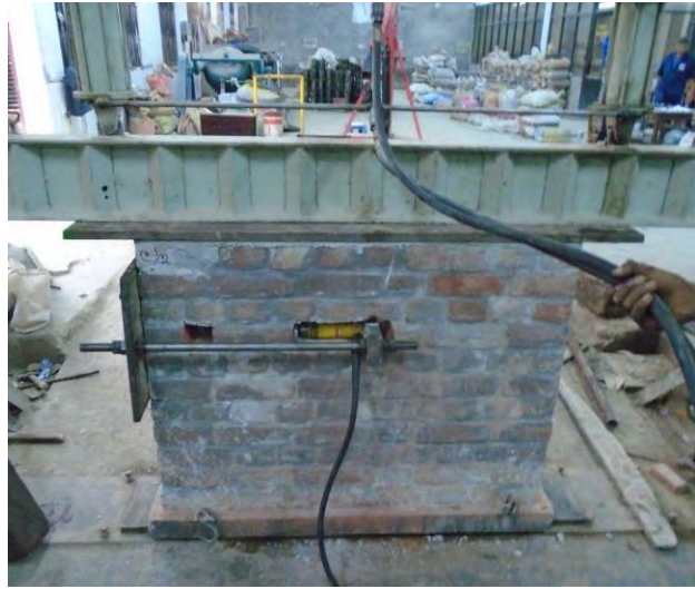
b. Shear test setup of clay burnt brick wall (C-1/2) with mortar thickness 1/2"
