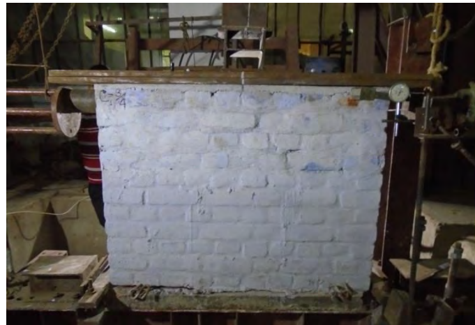
Figure 4.30 Final Crack Pattern of Specimen C1-3/4
