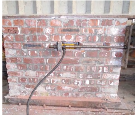
Figure 4.14 Failure Pattern of Shear Test
