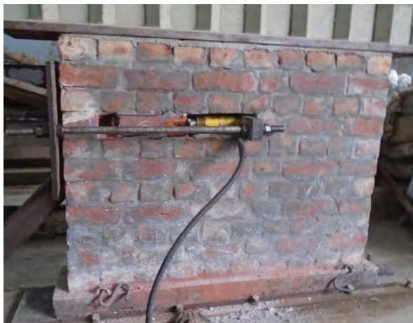
Figure 4.9 Failure Pattern of Shear Test Specimen C-1/2
