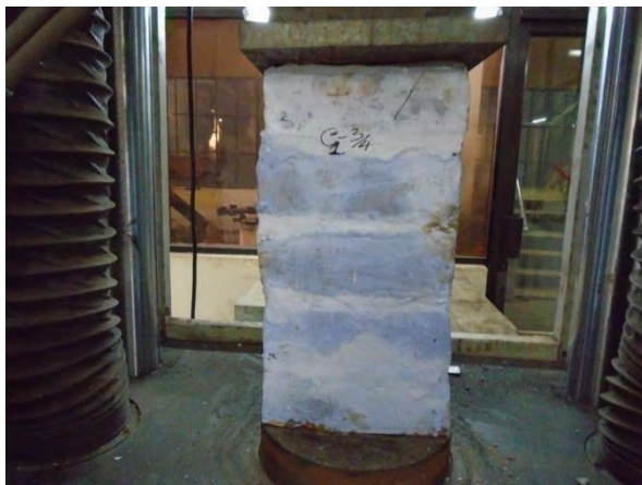
a. Appearance of first crack of prism C1-3/4
