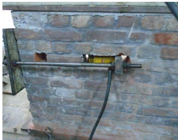
Figure 4.10 Failure Pattern of Shear Test Specimen C1-1/2
