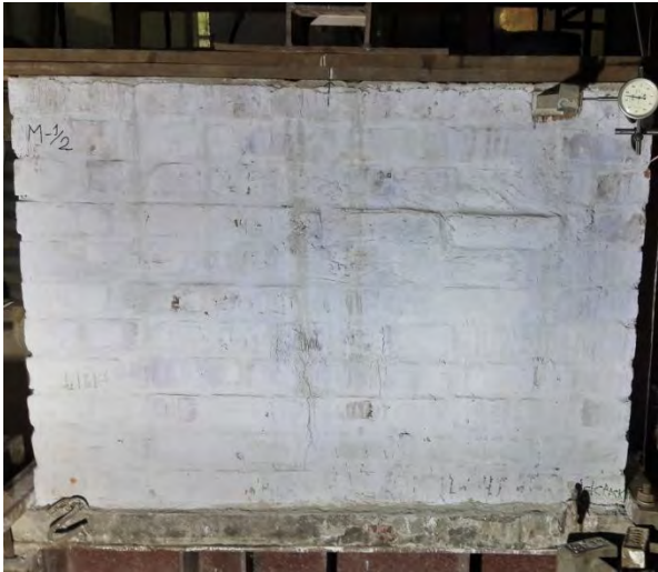
Figure 4.31 Initial Crack (Flexure) Patterns at Specimen M-1/2
