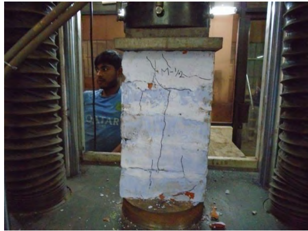
b. Ultimate crack of prism M-1/2
