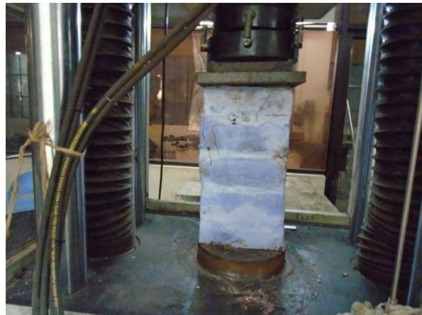
b. Ultimate crack of prism C1-3/4
