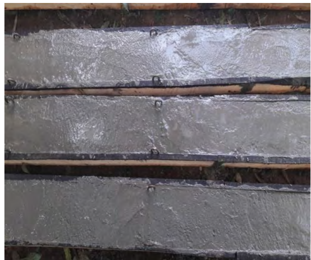
Figure 3.5 Casted Specimens with Formwork
