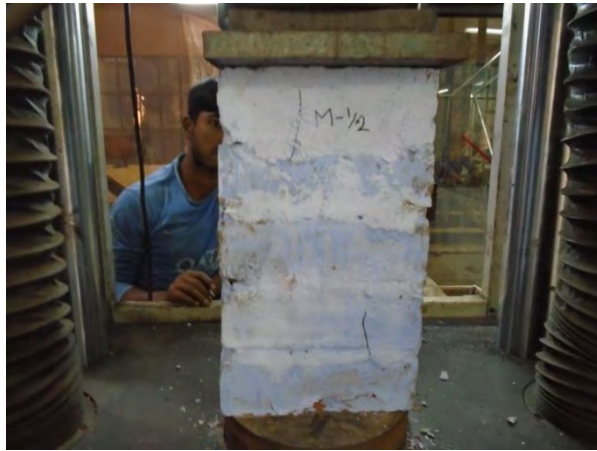
a. Appearance of first crack of prism M-1/2
