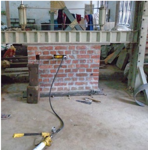
g. Shear test setup of machine made brick wall (M-3/4) with mortar thickness 3/4"
