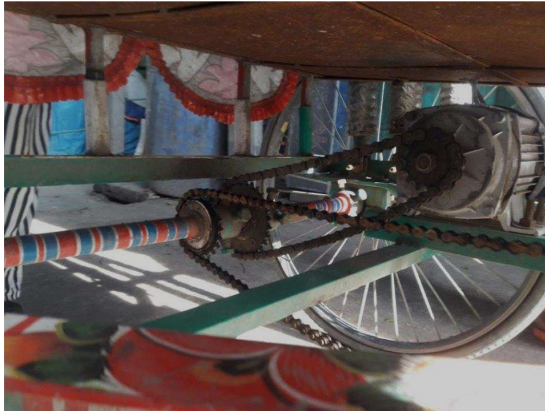
Figure 2.2 : BLDC motor inside the rickshaw
