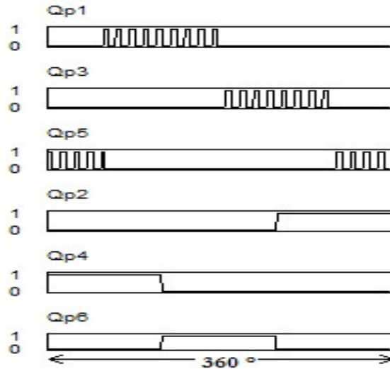
Figure 4.5: The switching pulses
