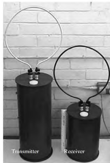
Fig. 2.7: Underwater transmitter and receiver using loop antenna [75].
